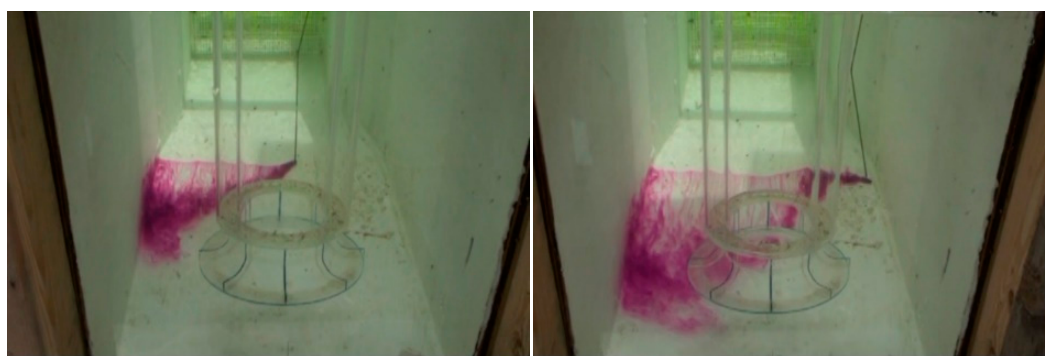
Figure 8. Injecting dye across the width of the pump bay shows a uniform and stable approach flow.
