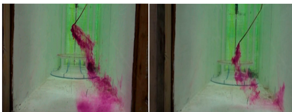
Figure 13. Flow instability and drifting behind the pump.
