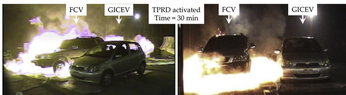
**Figure 6.** A fireball ignited by a controlled  $H_2$  release managed by a TRPD—Two different views of the front of the vehicles (left a default FCV, and right a classic and undamaged gasoline vehicle (GICEV)) [76].
