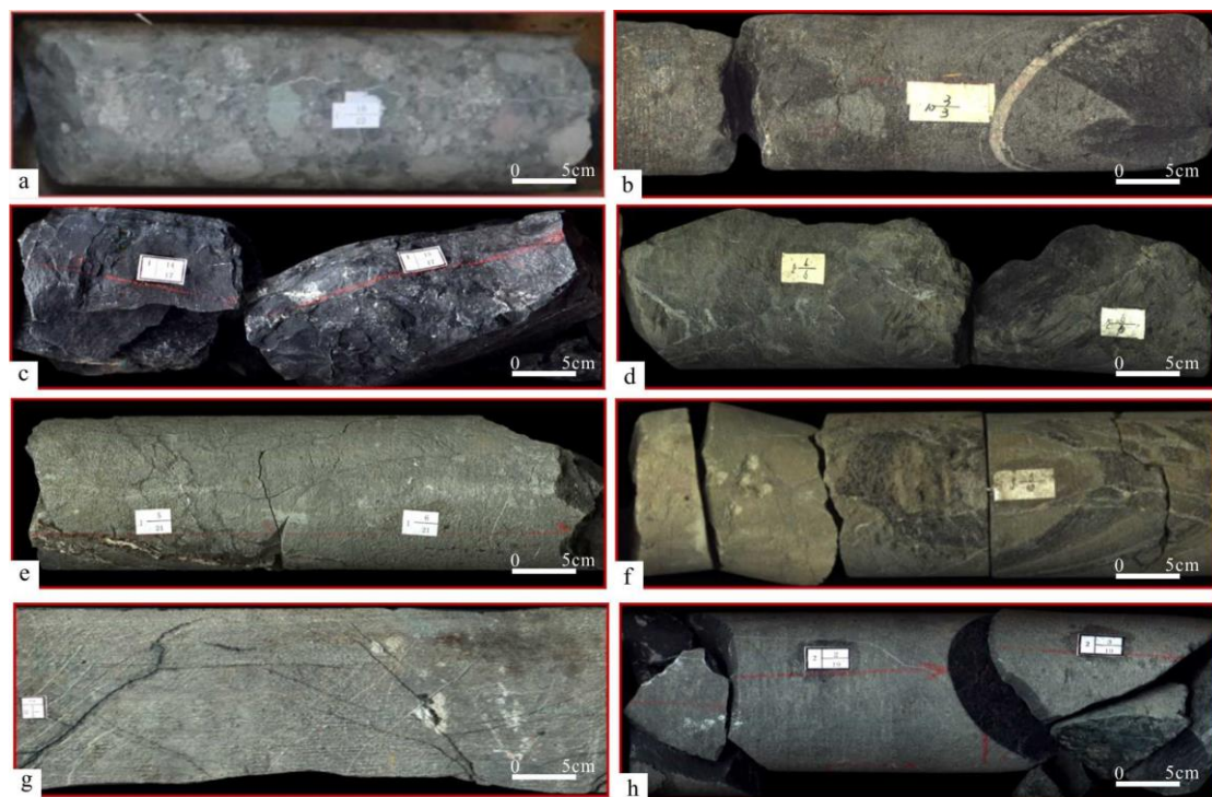
Figure 12. Photos showing the lithology of Carboniferous Formation in the Che 210 well block. (a) The volcanic breccia in the Che 210 well at 1447.5–1447.6 m. (b) The volcanic breccia in the Che 22a well at 1866.3–1866.5 m. (c) The tuff in the Chefeng 7 well at 1267.5–1267.7 m. (d) The tuff in the Che 40 well at 1377.7–1378.0 m. (e) The tuffaceous sandstone in the Che 211 well at 1176.6–1177.0 m. (f) The tuffaceous sandstone in the Che 44 well at 1600.9–1601.1 m. (g) The andesite in the Chefeng 7 well at 1350.2–1350.3 m. (h) The basalt in the Chefeng 7 well at 1350.4–1350.6 m.
