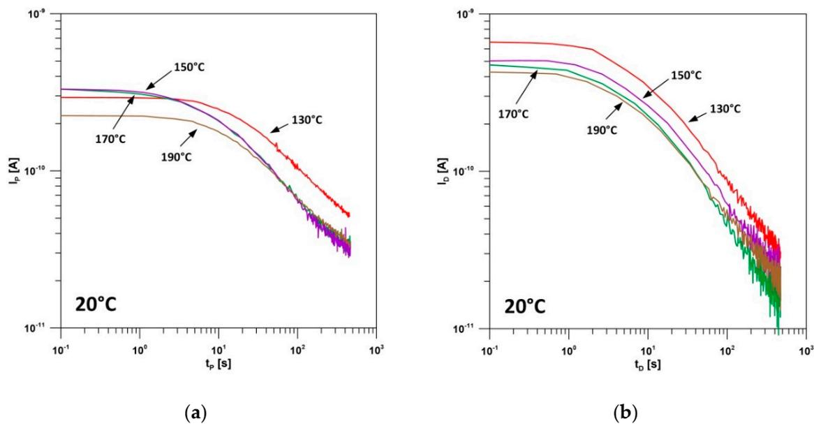
**Figure 12.** Characteristics of the polarization currents (a) and the depolarization currents (b) measured for unmoistened cellulose–aramid insulation samples for different degrees of initial ageing in the measurement temperature 20 °C.
