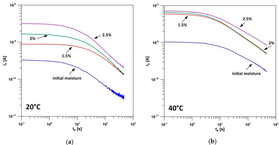
**Figure 8.** Characteristics of the polarization current of cellulose–aramid insulation sample with initial thermal ageing at 150 °C and with various moisture: (a) polarization currents in the measurement temperature 20 °C; (b) polarization currents in the measurement temperature 40 °C.
