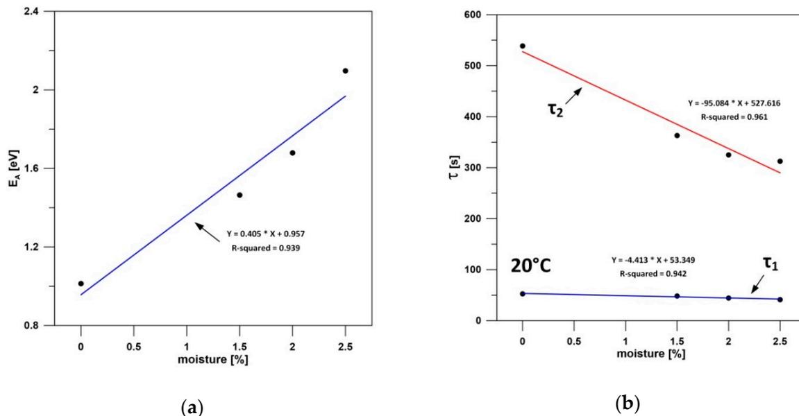
**Figure 11.** Dependence of the activation energy  $E_A$  (a) and dominant time constants  $\tau_1$  and  $\tau_2$  (b) on the degree of moisture for a selected non-aged cellulose–aramid insulation sample.
