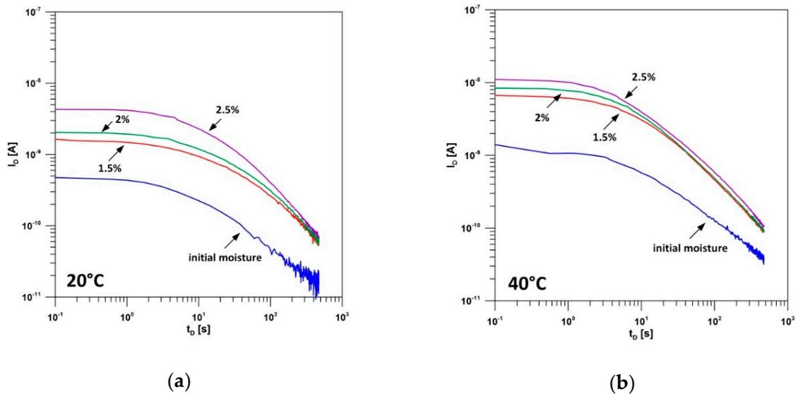
**Figure 9.** Characteristics of the depolarization current of cellulose–aramid insulation samples with initial thermal ageing at 150 °C and with various moisture: (a) depolarization currents in the measurement temperature 20 °C; (b) depolarization currents in the measurement temperature 40 °C.
