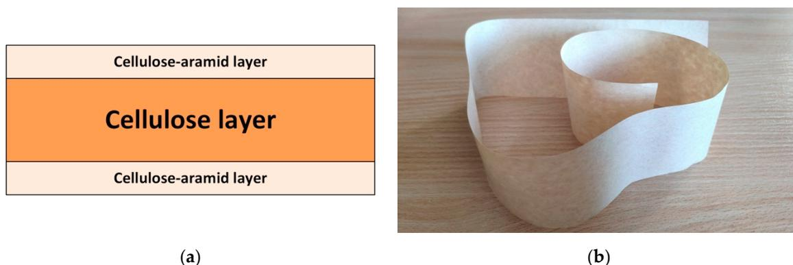
**Figure 1.** NOMEX<sup>®</sup>910 material structure: (a) cross-section; (b) photograph of a small sample.
