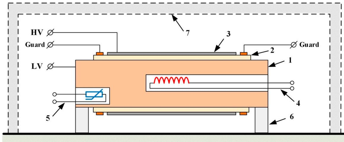
**Figure 3.** View of the measuring electrode system and the insulation sample studied: 1—a roll made of brass (LV—low potential electrode), 2—aramid–oil insulation sample, 3—metal foil (HV—high potential electrode), 4—heater, 5—temperature sensor, 6—insulator, 7—hermetic vessel plus thermal insulation.
