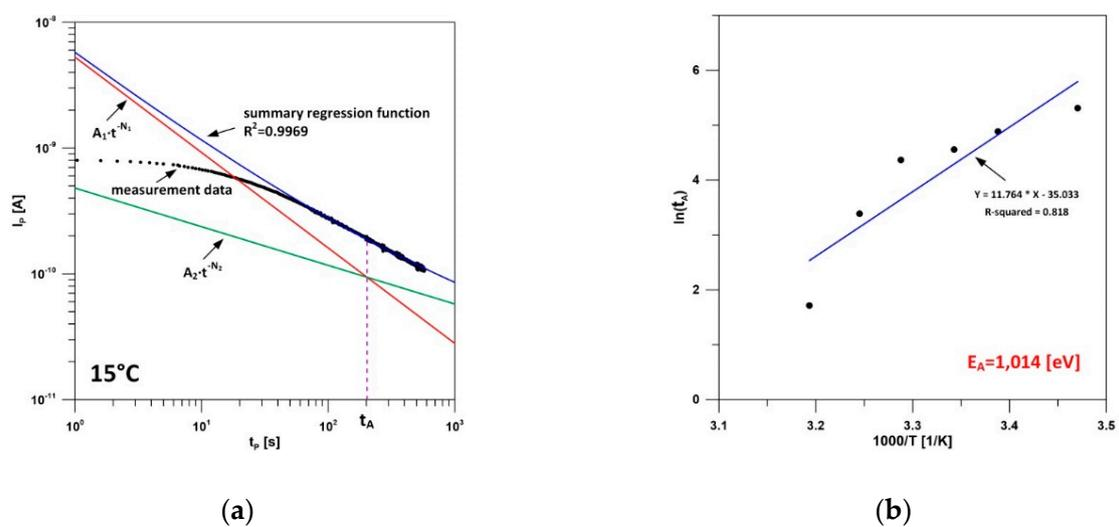
**Figure 10.** Method of fixing the activation energy  $E_A$  for a selected non-aged cellulose–aramid insulation sample with the smallest degree of moisture: (a) way of fixing  $t_A$  characteristic time from the polarization current; (b) Arrhenius graph.
