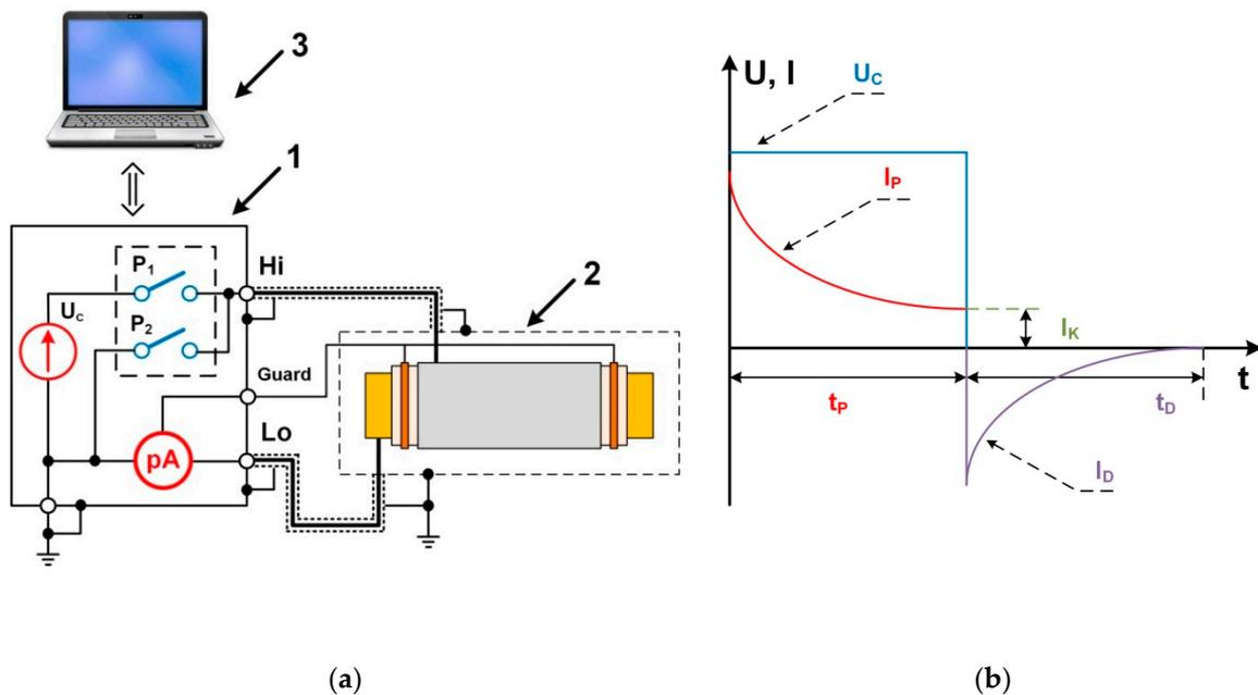
**Figure 5.** Diagnostics of the state of paper–oil insulation samples using the polarization and depolarization current analysis (PDC) method: (a) connections diagram; (b) time characteristics of currents and voltages. 1—measuring-switching system, 2—object being examined, 3—computer.
