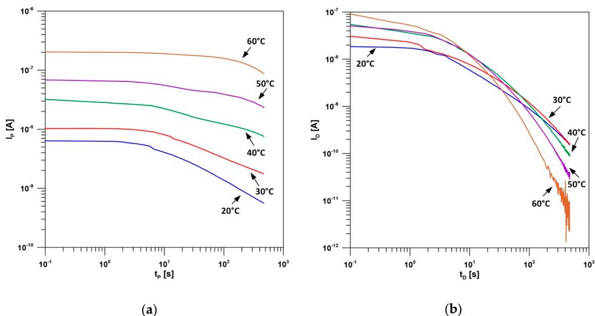
**Figure 6.** Effect of temperature on the characteristics of the PDC method for a selected cellulose–aramid insulation sample (non-aged with 1.5% moisture) mineral oil-impregnated: (a) polarization current; (b) depolarization current.
