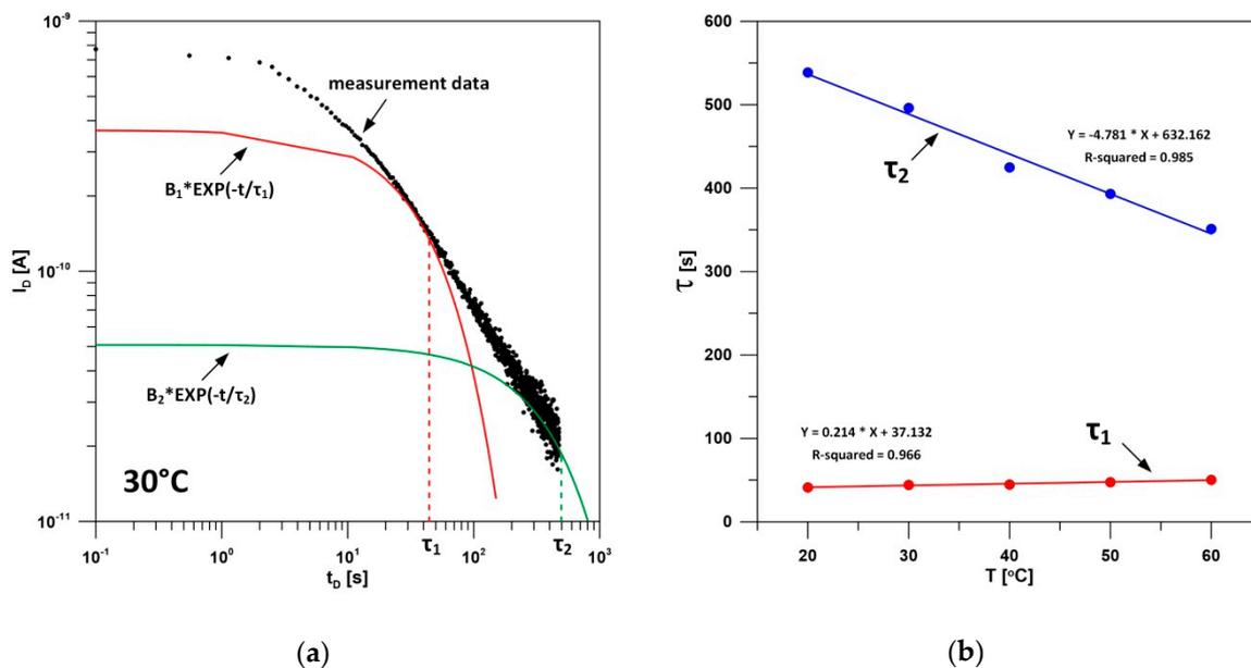
**Figure 7.** Analysis of time characteristics of the depolarization current by means of Debye regression function for a selected cellulose–aramid insulation sample (aged at 150 °C with the smallest moisture), mineral oil-impregnated: (a) depolarization current in the measurement temperature 30 °C; (b) temperature dependence of the dominant time constants for two relaxation processes.
