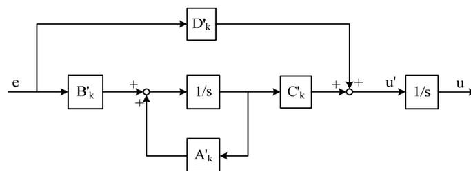
Figure 2. Special LPV controller that needs no modification.
