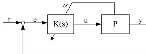
Figure 1. Linear Parameter Varying (LPV) control scheme.
