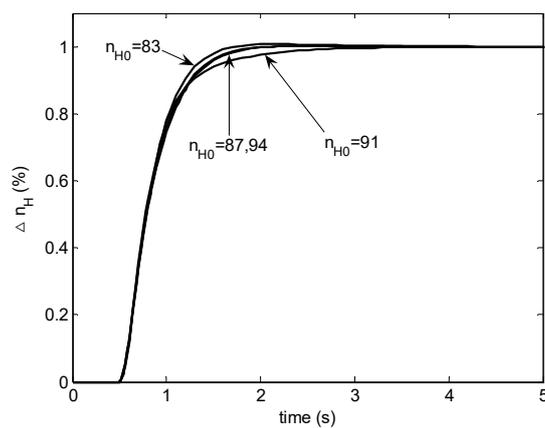
Figure 14. Step responses with the modified  $H_\infty$  LPV controller.
