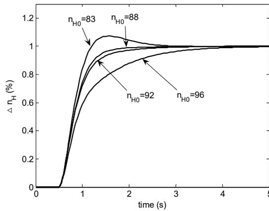
Figure 3. Step responses with a single proportional–integral (PI) controller.
