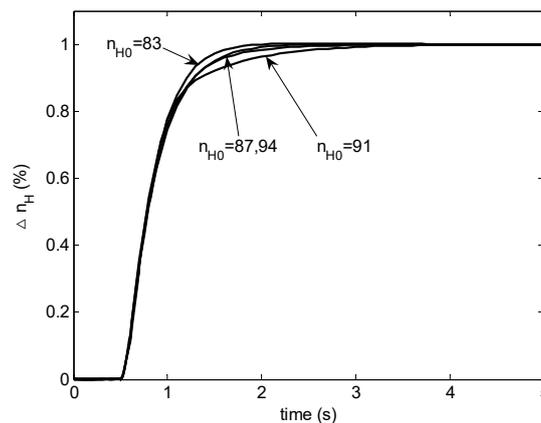
**Figure 16.** Step responses with the  $H_\infty$  LPV controller containing a pure integral part.
