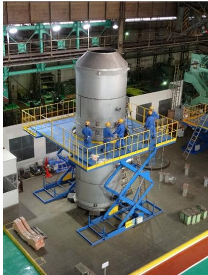
Figure 9. SO<sub>x</sub> scrubber using cyclone technology [105].
