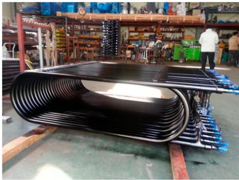
(a) Actual scale double pipe heat exchanger
