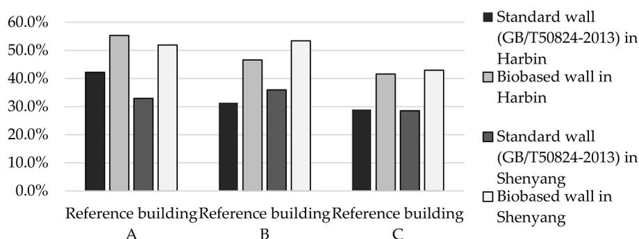
**Figure 7.** Reduction ratio of coal use of reference buildings with modified wall constructions in comparison with conventional residential buildings.
