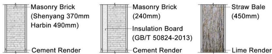
**Figure 3.** Wall construction of conventional wall (**left**), standard wall in GB/T50824-2013 (**middle**) and straw bale wall (**right**).
