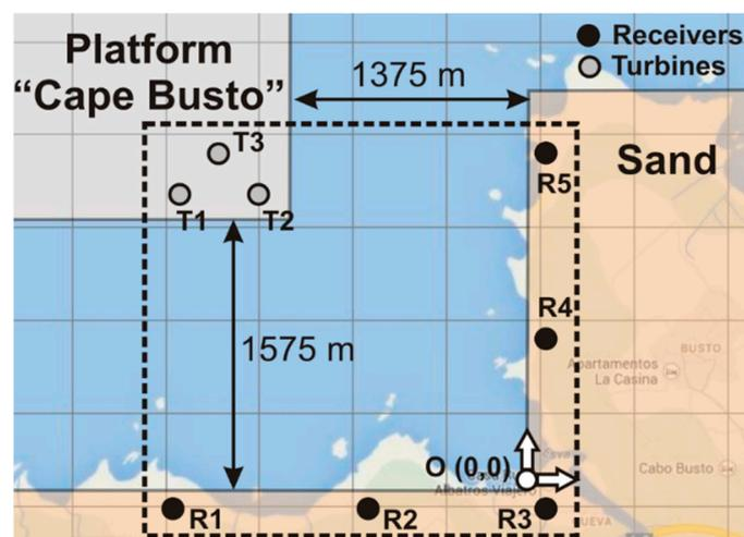
**Figure 4.** Sources and receivers' positions for the Cape Busto location.
