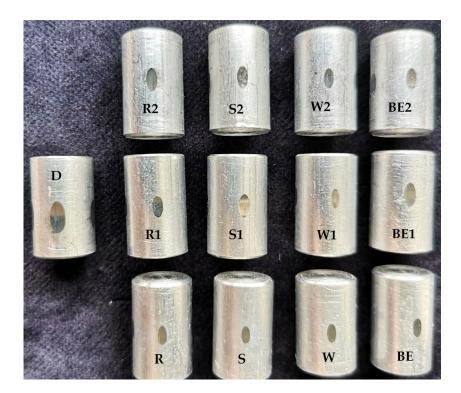
Figure 7. View of the signs of wear of selected samples lubricated with biofuels after tests.
