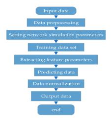
Figure 4. Wind speed prediction flow chart based on LSTM model.
