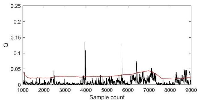
**Figure 9.** The  $Q$ -statistic of the EVT based on the proposed RPCA.
