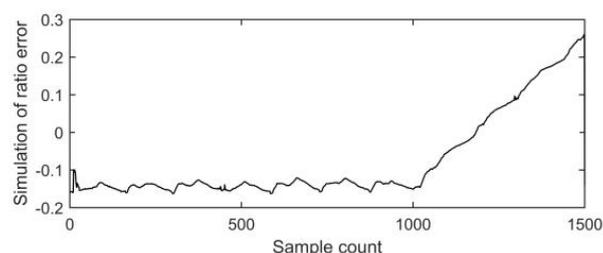
**Figure 3.** The ratio error of EVT phase-A with simulated fault.
