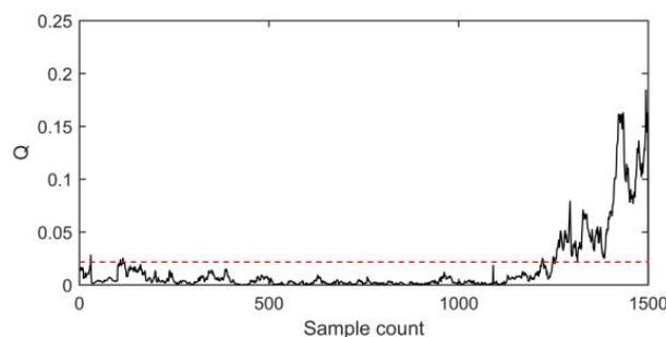
**Figure 4.** The  $Q$ -statistic of EVT based on the PCA model.
