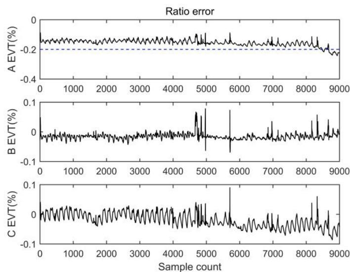
**Figure 8.** The ratio error of the EVT.
