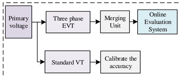
**Figure 1.** Schematic diagram of the field test. EVT: electronic voltage transformer. VT: voltage transformer
