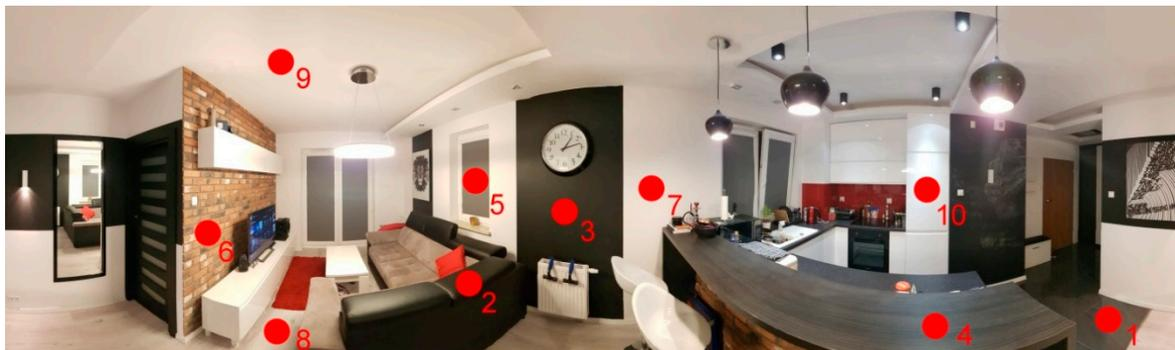
**Figure 4.** Layout of luminance measuring points in interior.
