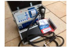
Figure 3. Exhaust gas analyzer with a measuring probe.
