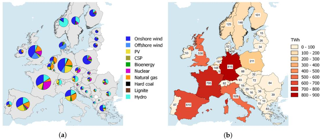
**Figure 3.** National capacity mix and electricity load of the investigated “large-scale RES” scenario for 2050 as defined by the e-Highway study [34]. Own illustration. (a) capacity mix; (b) electricity load.
