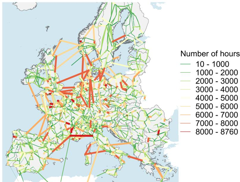
Figure 7. Frequency of line loading beyond 50% of the nominal capacity.
