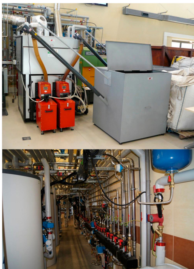
Figure 2. Experimental stand for biomass combustion with the biomass tank, feeder, Forster Heizkessel boiler and the Laboratory of Thermal Technologies (LTT) energy distribution system.
