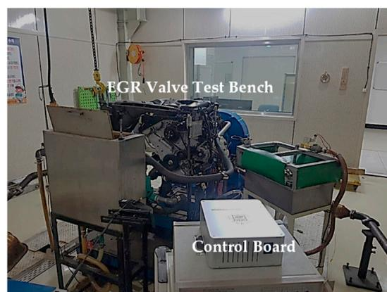
**Figure 9.** The EGR valve test bench and control board.
