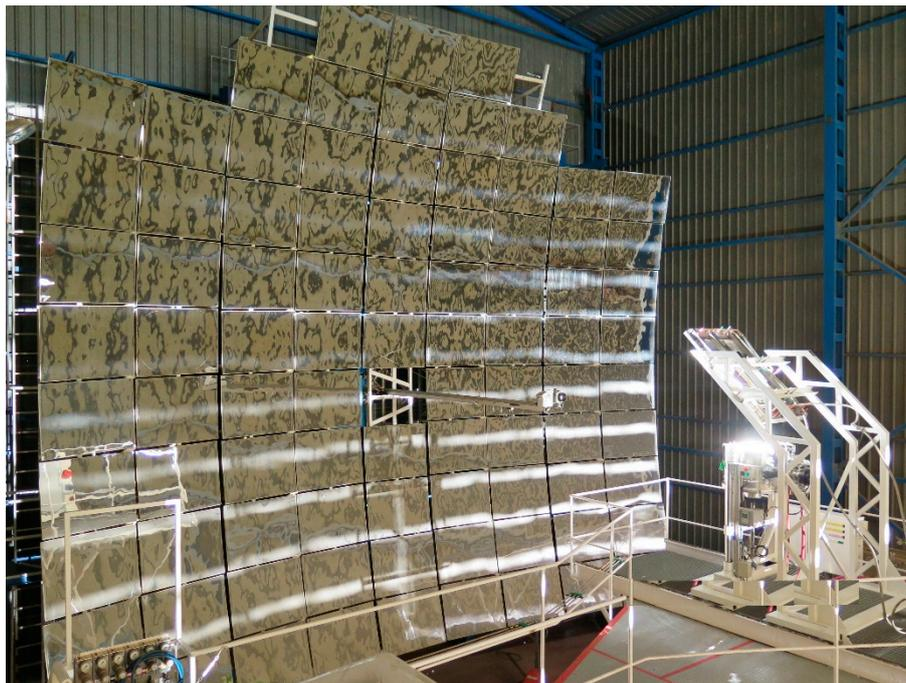
**Figure 1.** An indoor photo of the SF60 solar furnace, showing concentrator (left) and the 45°-tilted flat mirror (475 mm from the focal point) reflecting the concentrated solar radiation to the sample region below.
