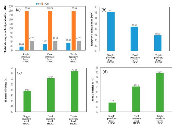
**Figure 3.** Electrical energy from GT, ST and heat production Q (**a**), energy self-consumption (**b**) and overall system thermal efficiency for the system with 1P, 2P, and 3P HRSG without (**c**) and with (**d**) inter-stage steam overheating.
