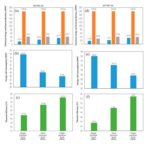
**Figure 4.** Electrical energy generation from GT, ST and heat production  $Q(\mathbf{a}, \mathbf{d})$ , energy self-consumption,  $(\mathbf{b}, \mathbf{e})$  and the overall system thermal efficiency  $(\mathbf{c}, \mathbf{d})$  for the system with 1P, 2P, and 3P HRSG with a steam regeneration system  $(\mathbf{a}-\mathbf{c})$  and with inter-stage superheating and regeneration of steam  $(\mathbf{d}-\mathbf{f})$ .
