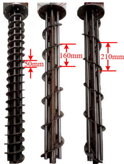
Figure 3. Heat transfer structure of heaters.
