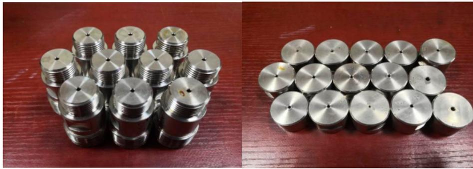
Figure 4. The physical diagram of OH self-excited oscillation nozzle.
