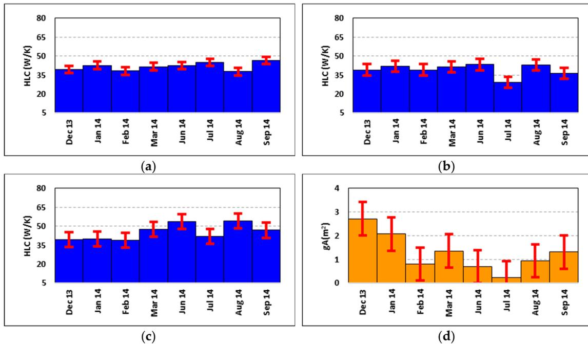
**Figure 12.** Results obtained using Model 21 for the data series of winter and summer in the first year. (a) HLC obtained using Model 21 as it is in Figure 10, (b) HLC obtained eliminating  $P_{PV}$  from node 2 in Model 21, (c) HLC using  $G_h$  instead of  $P_{PV}$  in Model 21, (d)  $gA$  using  $G_h$  instead of  $P_{PV}$  in Model 21.
