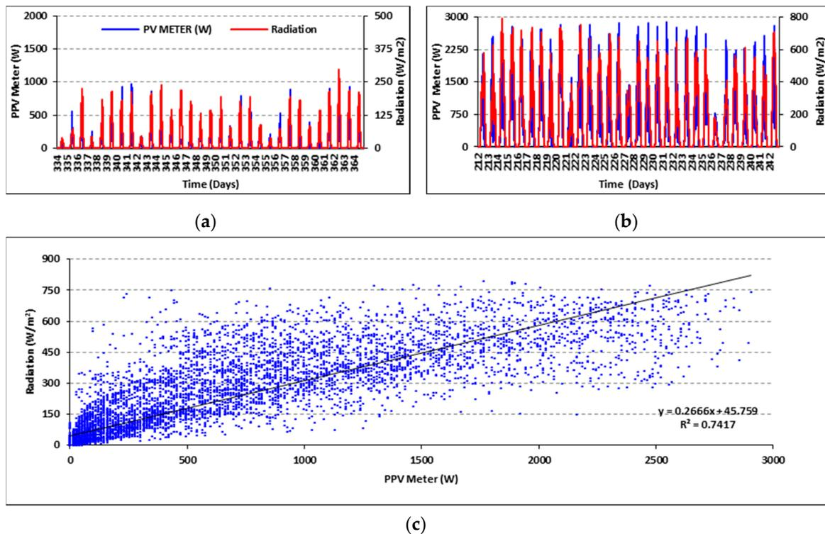
**Figure 2.** Electricity produced by the PV system vs. solar radiation measurements in Waddington, 30 km away from the building location: (a)  $P_{PV}$  meter vs. radiation, August 2014; (b)  $P_{PV}$  meter vs. radiation, December 2014; (c)  $P_{PV}$  meter vs. radiation, 2014 (all year).
