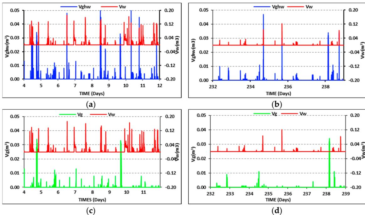
**Figure 3.** Estimation of unmeasured gas used for space heating ( $V_g$ ) from measured total ( $V_{ghw}$ ) and DHW ( $V_w$ ) gas used. Examples of typical months for summer and winter: (a)  $V_{ghw}$  vs.  $V_w$ , January 2014; (b)  $V_{ghw}$  vs.  $V_w$ , August 2015; (c)  $V_g$  vs.  $V_w$ , January 2014; (d)  $V_g$  vs.  $V_w$ , August 2015.
