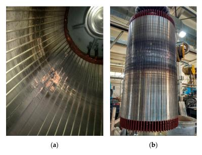
Figure 4. Effects of rubbing between rotor and stator due to eccentricity: (a) damage of the stator; (b) damage of the rotor.
