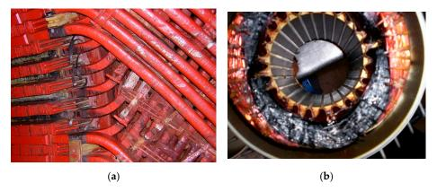
**Figure 2.** Stator winding faults: (**a**) short circuit in a high voltage winding; (**b**) short circuit in a low voltage winding.
