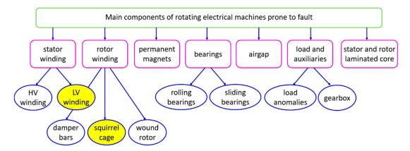
**Figure 1.** Main components of rotating electrical machines prone to fault, as divided into sections and subsections of this paper (from Section 4 to Section 10); in yellow, the subsections with a sub-subsection dedicated to power supply by electronic converter.
