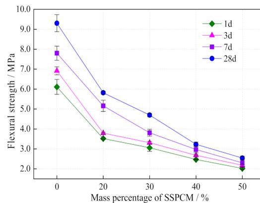
Figure 17. Flexural strength of SCTESM.
