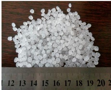
Figure 1. Low density polyethylene (LDPE).
