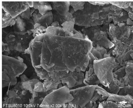
Figure 2. SEM image of flake graphite.
