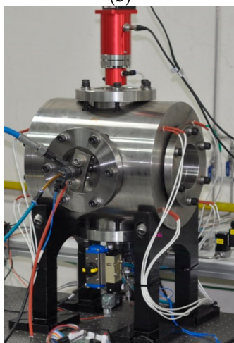
Figure 2. Optical setups for (a) the microscopic spray, (b) macroscopic spray visualizations, and (c) the constant volume chamber system.
