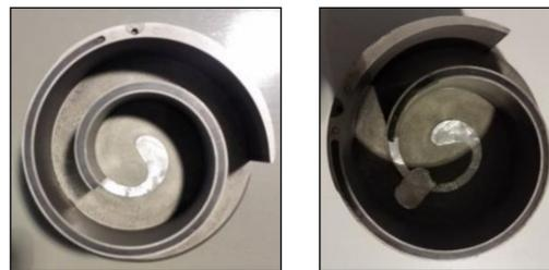
**Figure 7.** Cutting photos of intake chamber.
