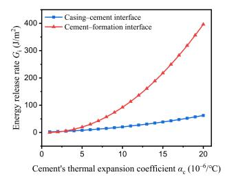
Figure 6. Evolution of the energy release rate at interfaces with cement's thermal expansion coefficient.
