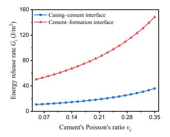
Figure 5. Effect of cement's Poisson's ratio on interfacial debonding.
