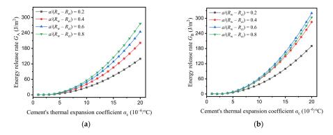
**Figure 10.** Evolution of the energy release rate at the radial crack tips with due to the thermal expansion coefficient of the cement: (**a**) crack tip A; (**b**) crack tip B.
