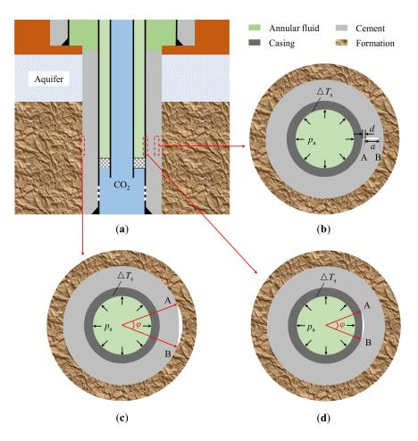
**Figure 1.** The schematic of a vertical injection well with defects in the wellbore barriers: (**a**) the vertical wellbore; (**b**) a radial crack in the cement; (**c**) an arc crack at the casing-cement interface; (**d**) an arc crack at the cement-formation interface.
