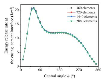
Figure A1. Energy release rate estimated with different element numbers.
