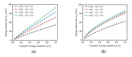
**Figure 8.** Energy release rate of a radial crack in cement as a function of the cement's Young's modulus: (a) crack tip A; (b) crack tip B.
