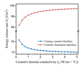
Figure 7. Effect of cement's thermal conductivity on the interfacial debonding.
