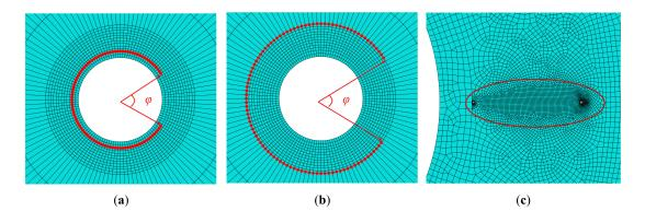
**Figure 2.** The meshes of the interfacial and radial cracks in the simulation: (**a**) the bonded nodes marked in red at the casing-cement interface; (**b**) the bonded nodes marked in red at the cement-formation interface; (**c**) the radial crack meshed with the refined mesh.
