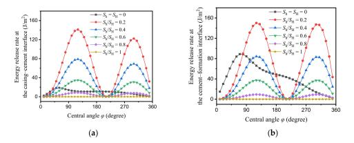
**Figure 12.** Impacts of in situ horizontal stresses on interfacial debonding: (**a**) crack at the casing-cement interface; (**b**) crack at the cement-formation interface.
