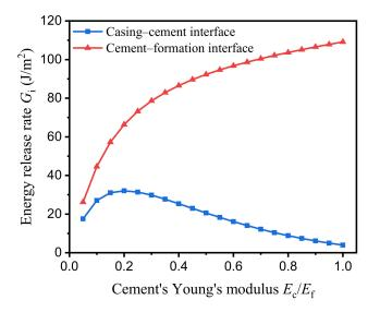
Figure 4. Variation of the energy release rates for interfacial debonding with the Young's modulus of cement.
