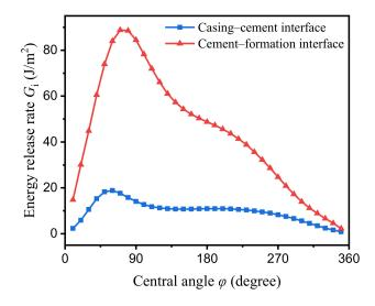
Figure 3. The energy release rate at the interfaces as a function of the central angle of the crack.
