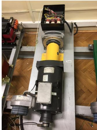
Figure 1. Tested generator with modified excitation system and driving DC machine.
