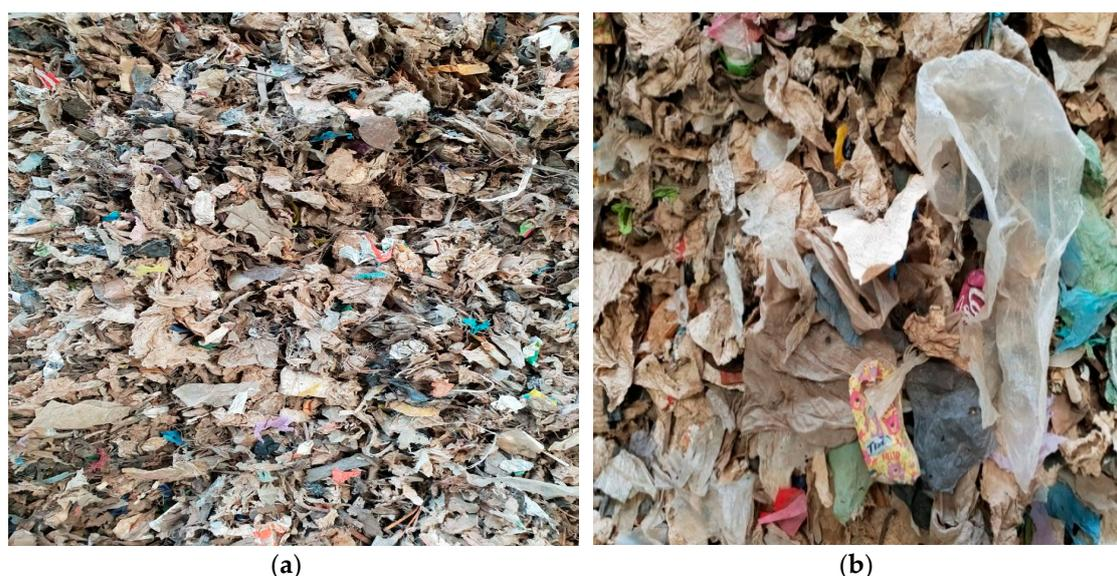
**Figure 2.** High-energy fractions separated from the CLO: (a) after the Zig-Zag separator (M-1); (b) after the NIHOT (M-2) separator.
