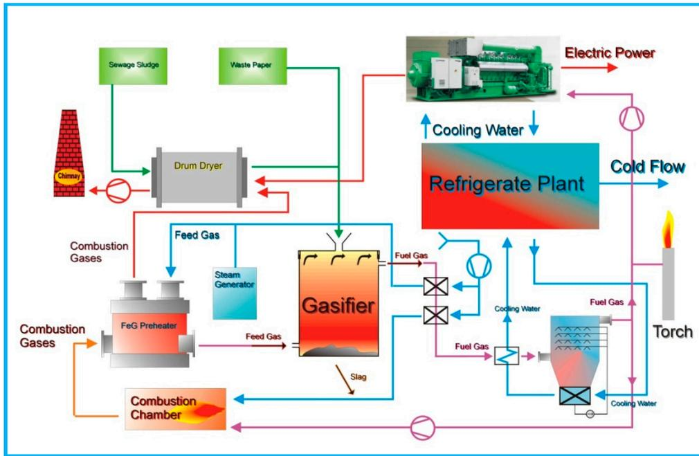
**Figure 17.** A proposal of a semi-industrial high-temperature biomass gasification installation for power generation design by KTH/GUT research group. The key component of the system is the FeG Preheater which produces a high-temperature feed gas.
