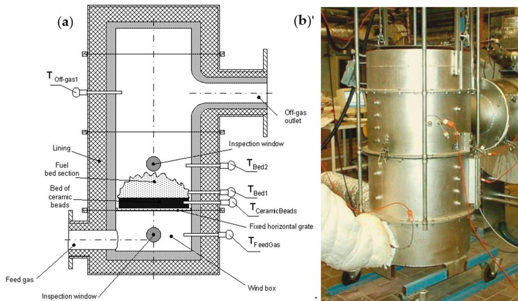
**Figure 6.** Side view of an updraft gasifier ( $T_{\text{Feed Gas}}$ —temperature of preheated feed gas,  $T_{\text{Bed1}}$ ;  $T_{\text{Bed2}}$ —reacting fixed-bed, fuel gas  $T_{\text{Off-gas1}}$  and ceramic beads  $T_{\text{Ceramic Beads}}$ ) (a), and batch type slag reactor HiTAG/HiTSG (b).
