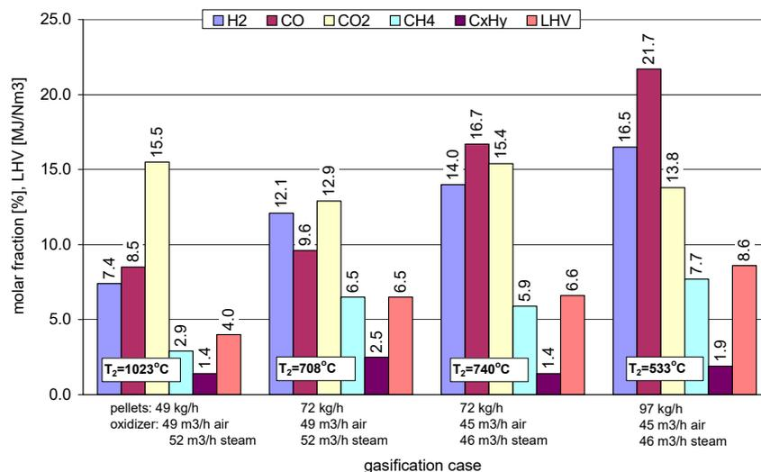
**Figure 15.** Composition of fuel gas and its LHV for different conditions of continuous HTAG with a preheated mixture of air and steam as the feed gas (experimental results).
