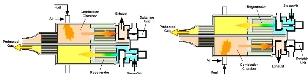
**Figure 2.** Concept of a high-temperature air/steam ceramic regenerator with a high-frequency alternating flow (with about 10–30 s for each mode) developed by Mochida and Hasegawa [5].
