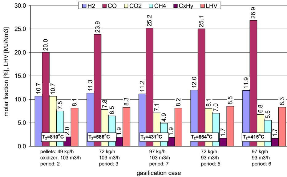
**Figure 12.** Composition of fuel gas and its LHV for different conditions of continuous HiTAG and preheated air as the feed gas (experimental results).
