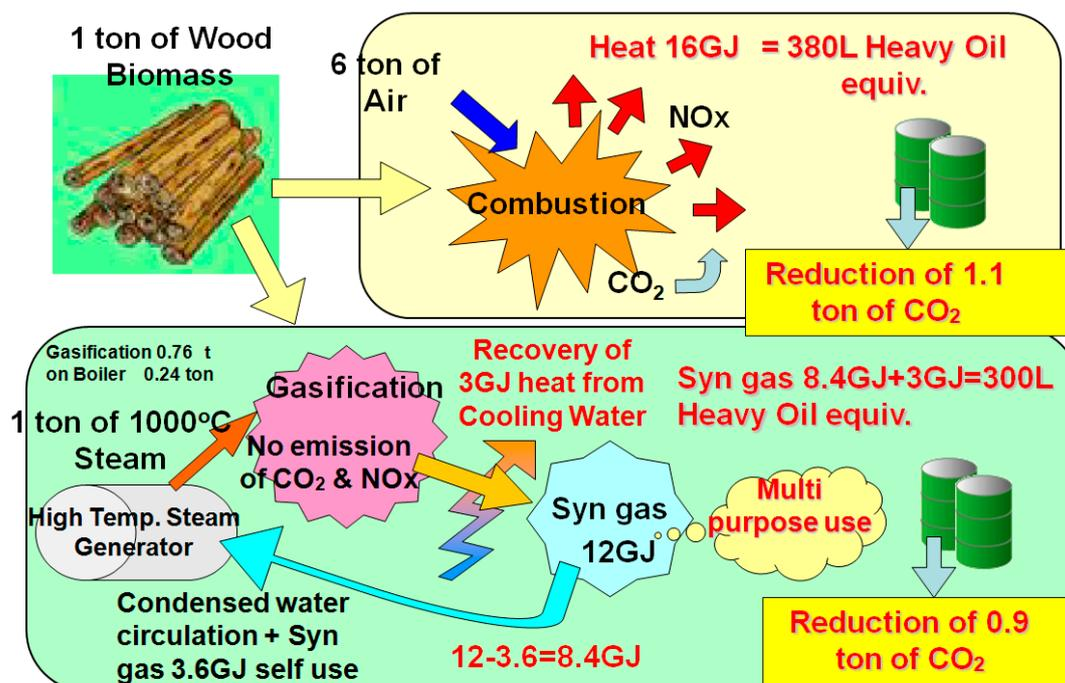
**Figure 16.** Example of effective utilization of biomass energy (Combustion and Gasification). Comparison of two methods: direct combustion (**top**) and gasification (**bottom**) shows a significant reduction of harmful pollutants.
