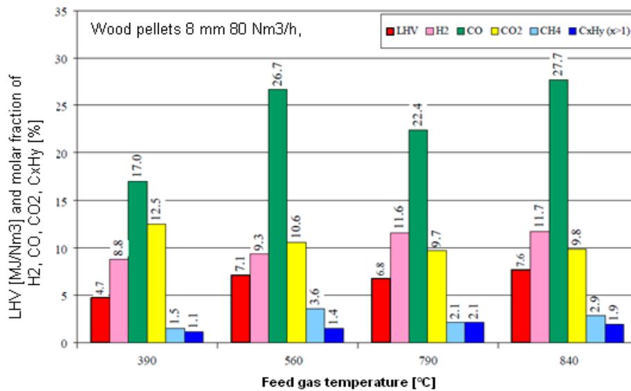
**Figure 13.** Influence of temperature of the feed gas on the average values of LHV and composition of dry fuel gas. Average values are taken from Phase II for batch type gasification 20 kg of 8 mm wood pellets.
