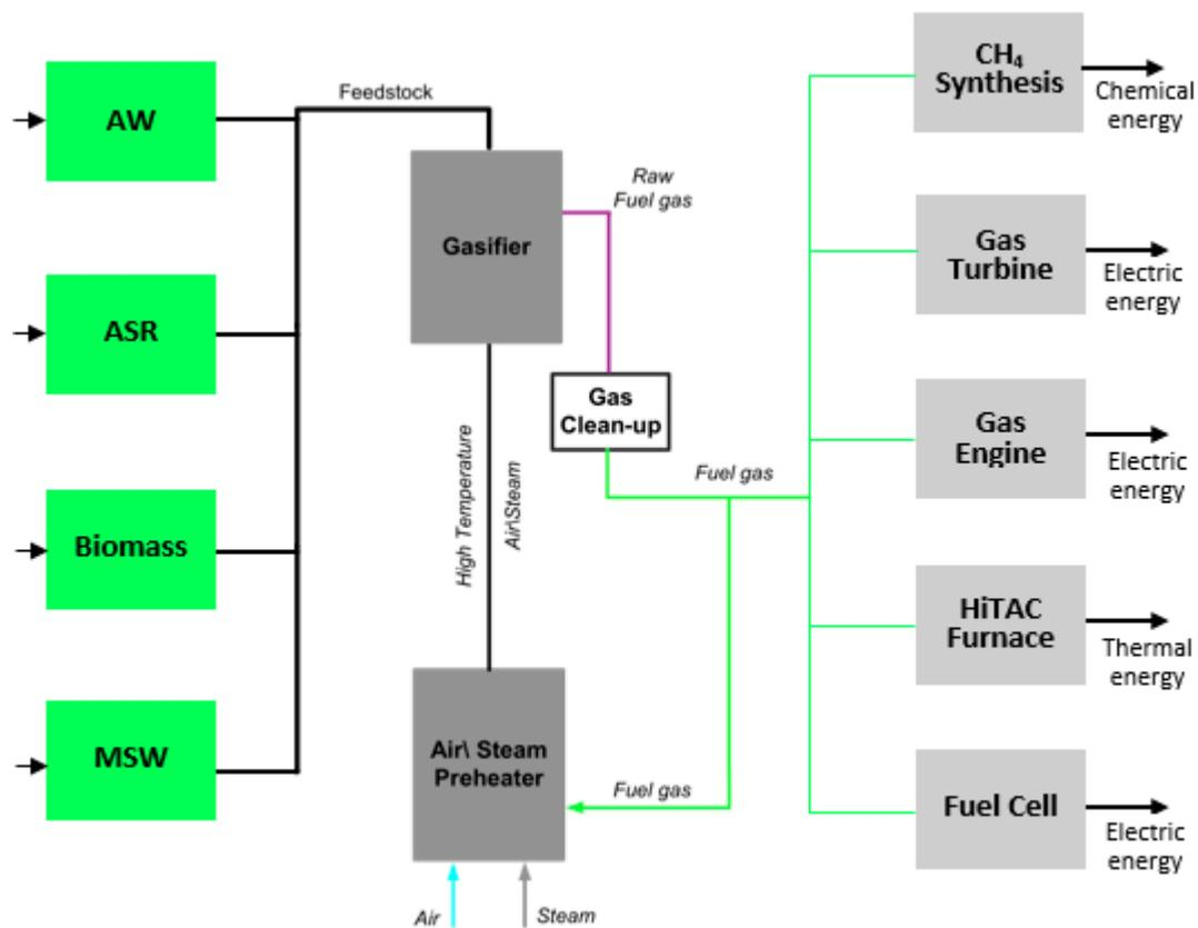
**Figure 5.** General schematics of HiTAG/HiTSG plant for different utilization alternatives of the fuel gas obtained from biomass and waste (AW—Animal waste; ASR—Automotive shredder residues; MSW—Municipal solid waste). High calorific gas produced in the process can be used as fuel gas in energy generation based on turbine engines, furnaces, or fuel cells.
