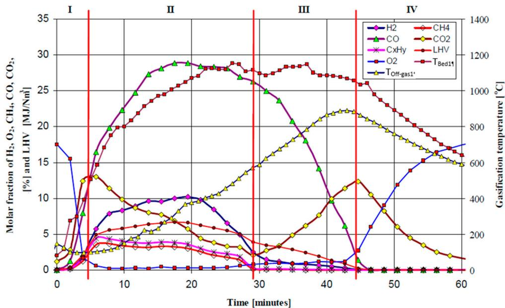
**Figure 9.** Changes of the fuel gas composition (H<sub>2</sub>, CO, CO<sub>2</sub>, CH<sub>4</sub>, C<sub>x</sub>H<sub>y</sub>, O<sub>2</sub>), LHV, gasifier bed temperature (T<sub>bed1</sub>) and the exiting fuel gas temperature (T<sub>off-gas1</sub>), versus gasification process time. Feed gas conditions: 50 Nm<sup>3</sup>/h of air preheated up to 350 °C (gasification 20 kg of 12 mm wood pellets).
