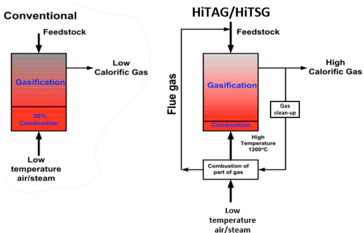
**Figure 4.** Comparison between conventional and HiTAG/HiTSG gasification. In the conventional system, the process involves lower temperatures (approx. 600–700 °C) and produces a low-calorific gas polluted with tars, ash, or even dioxin and furans. On the other hand, in the HiTAG/HiTSG system, ceramic regenerator allows obtaining high temperatures of the feed gas (flue gas) which produces high calorific and cleaner gas.
