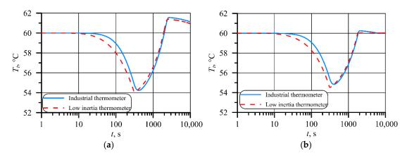
**Figure 10.** Temperature variations of the industrial thermometer and fast response thermometer obtained for the following PID controller settings: (a)  $K_p = 5.0$  W/K, the integral gain  $K_i = 1$  s<sup>-1</sup>, and the derivative gain  $K_d = 2$  s, (b)  $K_p = 1640$  W/K, the integral gain  $K_i = 100$  s<sup>-1</sup>, and the derivative gain  $K_d = 10$  s.
