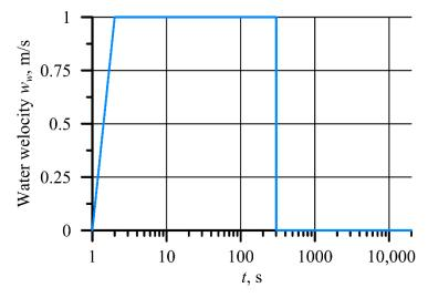
Figure 8. Water velocity in the tank feed tube.
