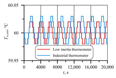
Figure 13. Temperature variations of the water temperature for low inertia and industrial thermometer as a function of time.
