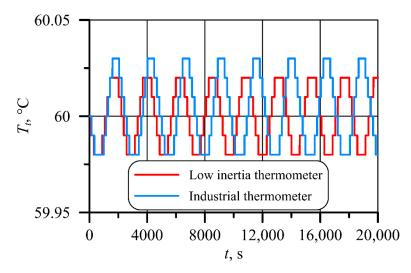
Figure 12. Temperature variations of the low inertia and industrial thermometer as a function of time.
