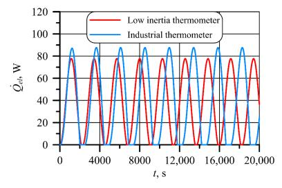
Figure 14. Electric heater power oscillations during PID control process.
