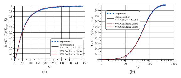
**Figure 6.** The time response of the industrial thermometer; (**a**) linear time coordinate, (**b**) logarithmic time coordinate.
