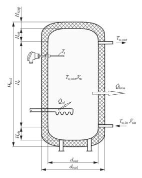
**Figure 1.** Hot water storage tank;  $H_{eh}$ —the height of tank elliptical head,  $H_c$ —the height of cylindrical part of the container,  $H_{iso}$ —the height of tank thermal insulation,  $d_{out}$ —outer diameter of the water storage tank,  $d_{isol}$ —outer diameter of thermal insulation,  $V_w$ —tank capacity,  $\dot{V}_{str}$ —water volume flow rate, m<sup>3</sup>/s.
