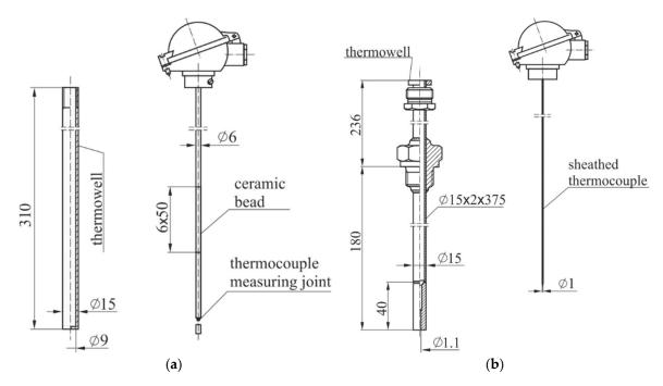
Figure 4. Thermometers used to measure the water temperature: (a) classic industrial thermometer, (b) innovative in-house design of the thermometer with small times constant.
