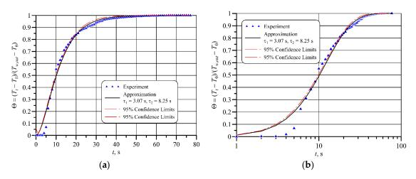
**Figure 7.** The time response of the fast-response thermometer; (**a**) linear time coordinate, (**b**) logarithmic time coordinate.
