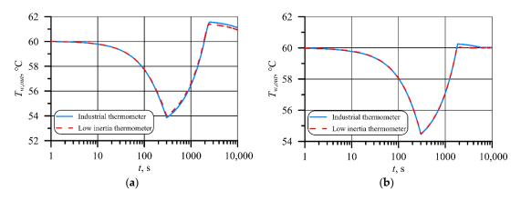
**Figure 11.** Changes in water temperature in the water volume heater obtained for the following PID controller settings: (a)  $K_p = 5.0$  W/K, the integral gain  $K_i = 1$  s<sup>-1</sup>, and the derivative gain  $K_d = 2$  s, (b)  $K_p = 1640$  W/K, the integral gain  $K_i = 100$  s<sup>-1</sup>, and the derivative gain  $K_d = 10$  s.
