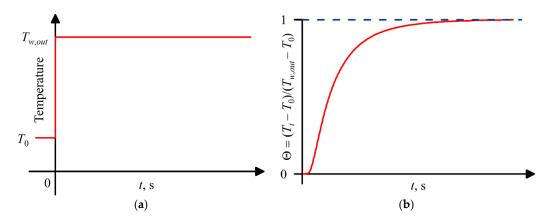
Figure 5. Stepwise increase in the temperature of the fluid (a) and the thermometer transient response (b).
