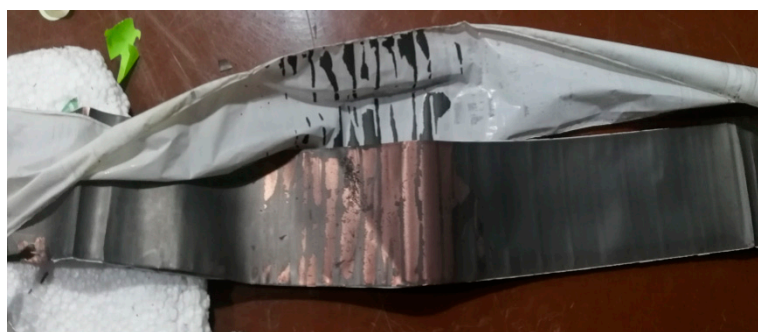
Figure 7. NCM811 battery disassembled after 1 C overdischarge.
