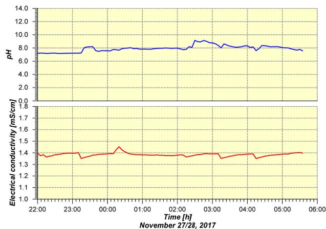
**Figure 5.** Variability of pH and EC during pumping in the CH PIG-1 borehole on 27–28 November 2017.
