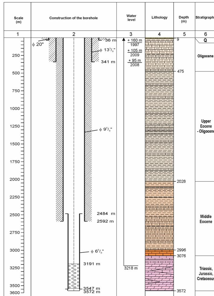
Figure 3. Construction of the CH PIG-1 borehole (based on [32], modified).
