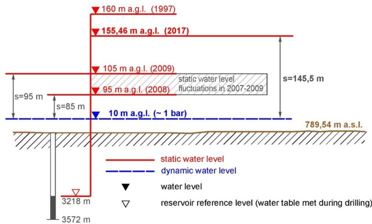
Figure 6. Static and dynamic water levels in the CH PIG-1 well.
