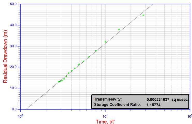
**Figure 8.** Diagnostic chart—pressure recovery after the second phase of the hydrodynamic test in the CH FIG-1 borehole.
