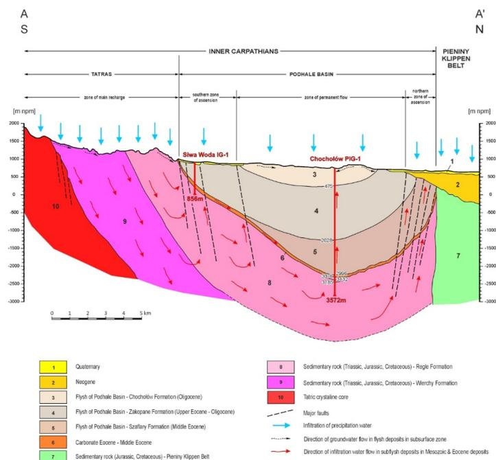
Figure 2. Geological profile of the CH PIG-1 borehole (based on [31], modified).
