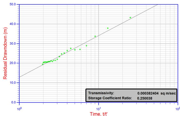
Figure 7. Diagnostic chart—pressure recovery after the first phase of the hydrodynamic test in the CH PIG-1 borehole.
