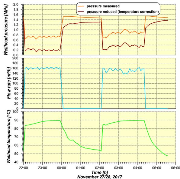
**Figure 4.** Variability of the flow rate, wellhead pressure, and temperature during pumping in the CH PIG-1 borehole on 27–28 November 2017.
