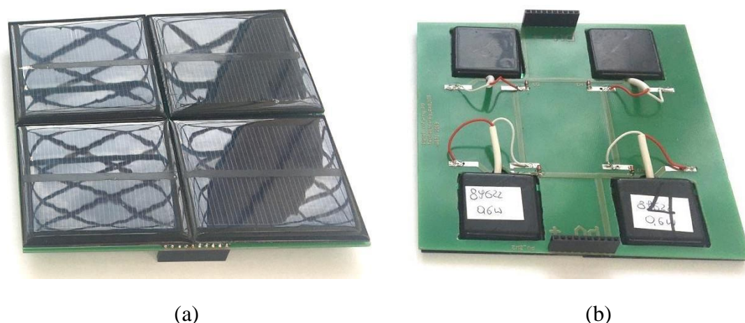
Figure S4. View of assembled PCB of first demonstrator- photovoltaic cells in a system of 40 cells connected in series in parallel in a 2 \times 10 \times 2 system: (a) page of elements; (b) print page.
