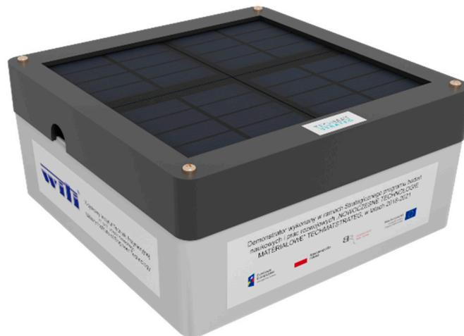
**Figure 2.** Photograph of a constructed demonstrator of an energy storage system based on silicon solar cells and supercapacitors [19].
