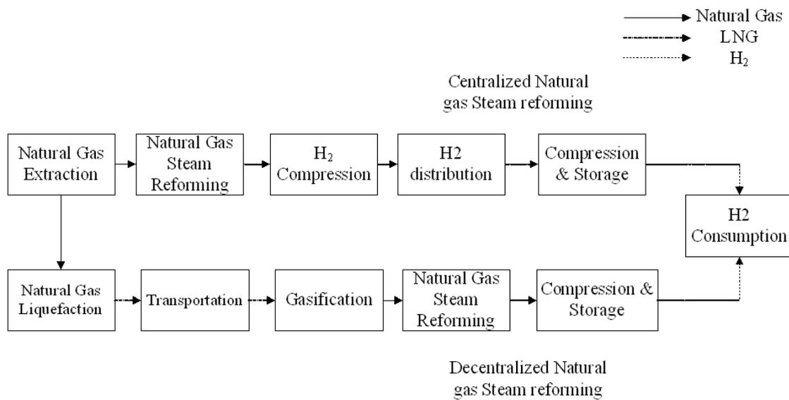
**Figure 4.** Hydrogen production process via natural gas steam reforming, centralized and decentralized forms.
