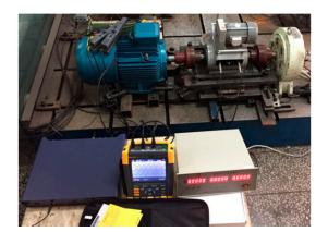
**Figure 17.** Test platform of 12/8 pole SRM is established, to verify the reliability of the calculation method and the accuracy of the calculation results.
