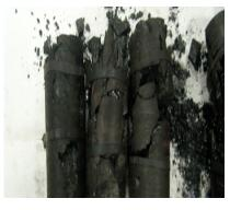
Figure 5. Failure pattern of coal samples.
