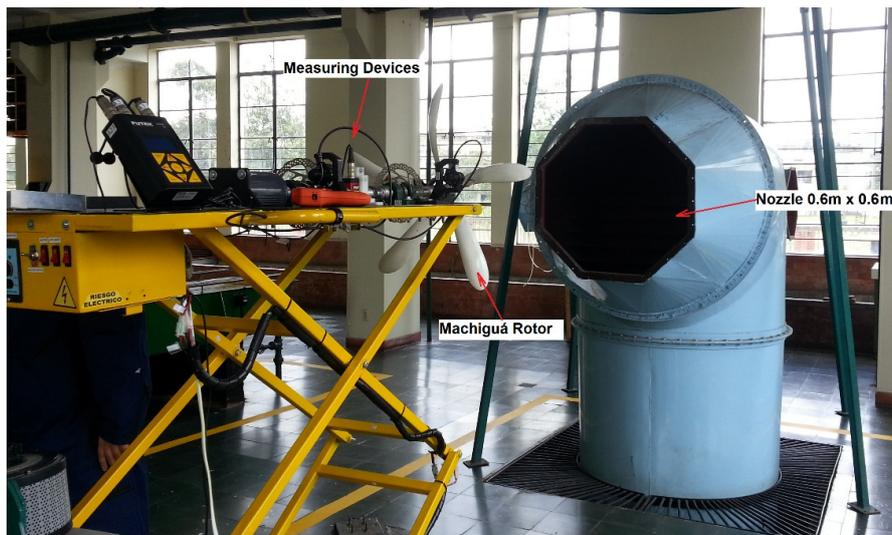
Figure 5. Experiment arrangement.
