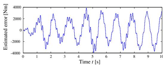
Figure 13. Estimated error of  $H_\infty$  observer at with white noise.
