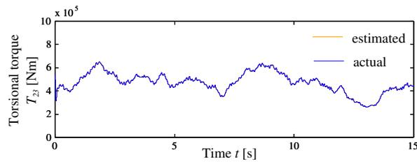
(d) Estimated result of torsional torque with  $H_\infty$  observer.
