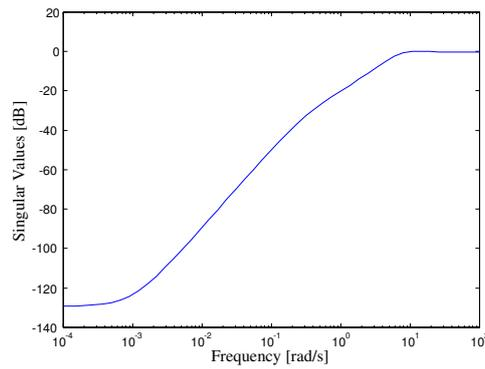
(b) Weighting function of high-pass filter characteristics for noise ( $W_2$ ).
