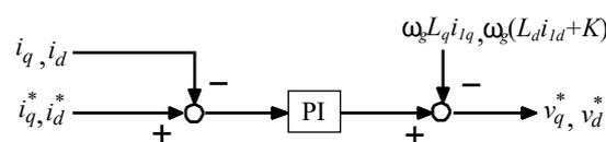
**Figure 4.** Generator side converter control system.
