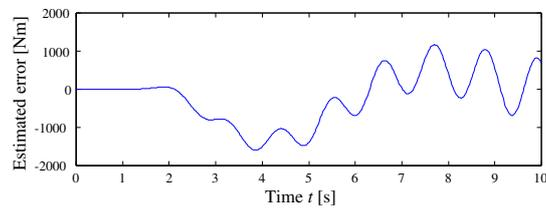
Figure 11. Estimated error of  $H_\infty$  observer at parameter error  $-20\%$ .
