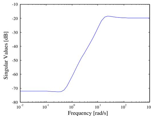
(b) Weighting function for suppress resonance ( $W_4$ ).
