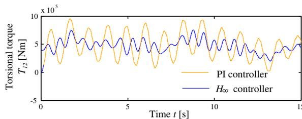
**(b)** Torsional torque  $T_{12}$ .
