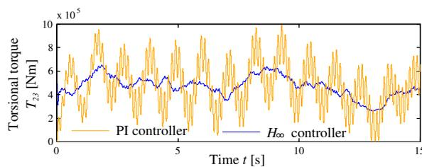
**(c)** Torsional torque  $T_{23}$ .
