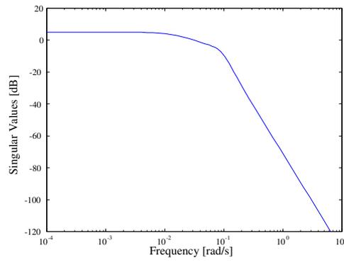
(a) Weighting function of low-pass filter characteristics for parameter error ( $W_1$ ).
