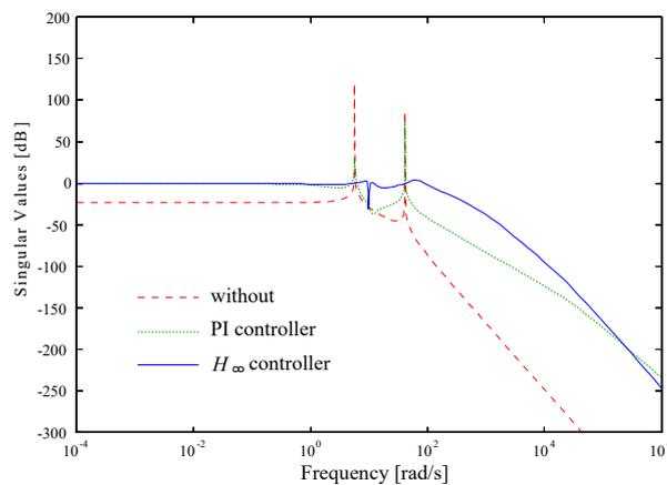
Figure 3. Frequency response of the shaft system.
