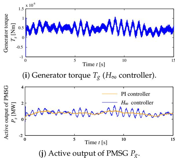
Figure 16. Simulation results in Proportional-Integral (PI) control and  $H_\infty$  control.
