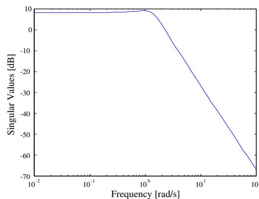
(a) Weight function for steady-state deviation removal for command value tracking ( $W_3$ ).
