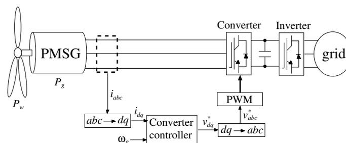
**Figure 1.** Configuration of power conversion control system of permanent magnet synchronous generator (PMSG) wind turbine.
