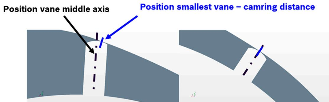
**Figure 4.** Variable contact point due to different radii of cam ring and vane tip.
