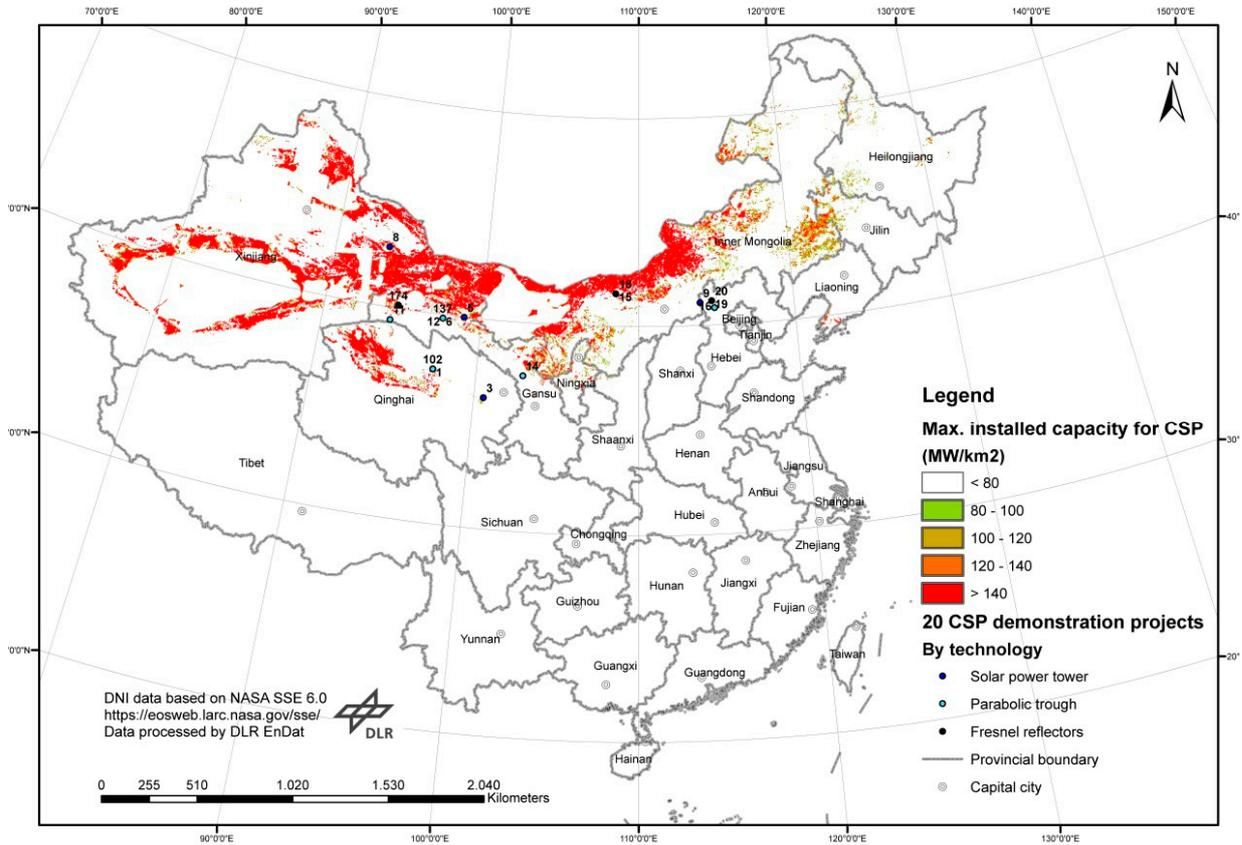
**Figure S3.** Maximum installable CSP capacity per km<sup>2</sup> and distribution of 20 demonstration CSP projects by technology in China.
