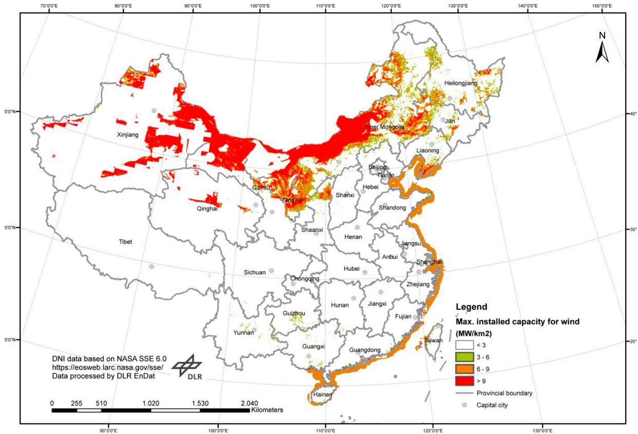
**Figure S1.** Maximum installable wind power capacity per km<sup>2</sup> over 4 m/s threshold in China.
