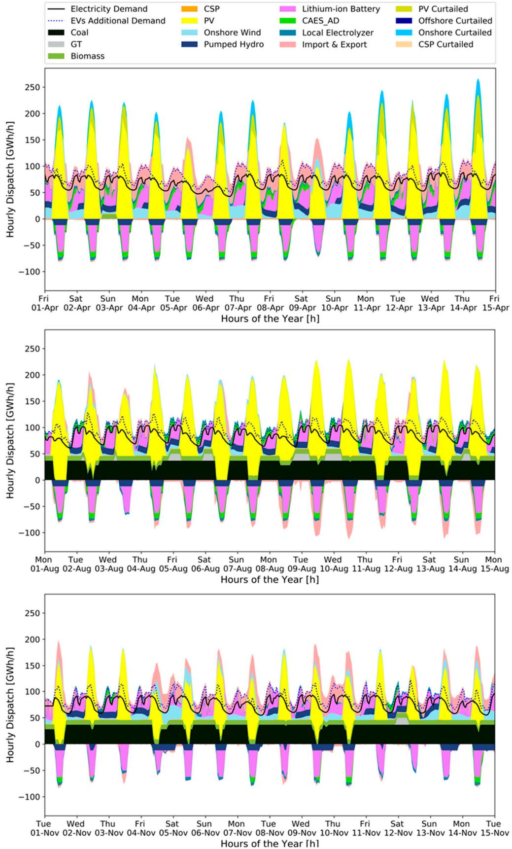
**Figure S11.** Typical hourly generation for each form of technology, export and charge (-), import and discharge (+) to meet power demand in Hebei in April, August and November in 2050.
