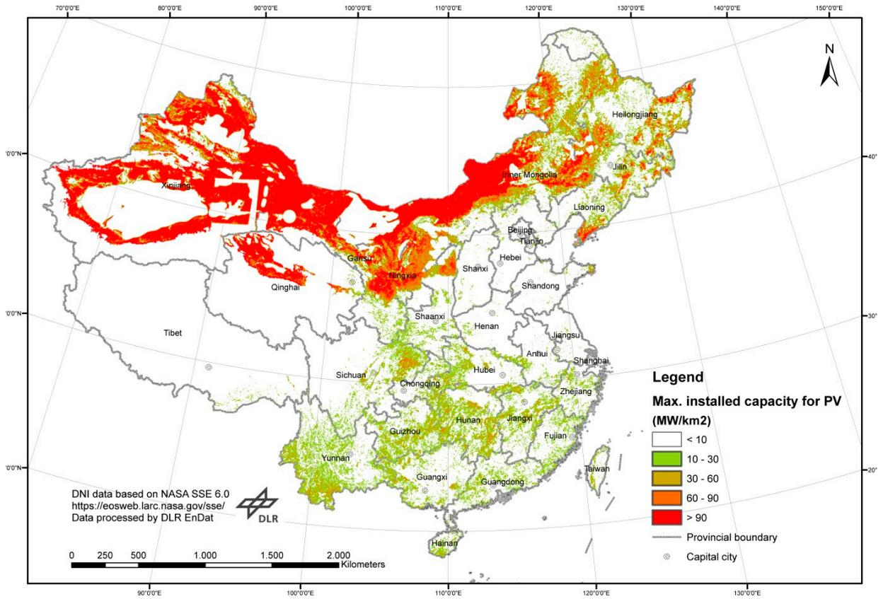
Figure S2. Maximum installable PV capacity per km<sup>2</sup> in China.
