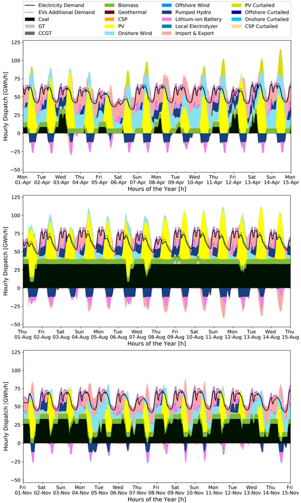
**Figure S7.** Typical hourly generation for each form of technology, export and charge (-), import and discharge (+) to meet power demand in Hebei in April, August and November in 2030.
