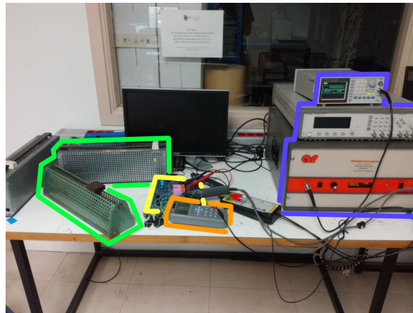
Figure 11. Photograph of the experimental setup for conducting the described RF test. In this setup, the input waveforms were generated using a signal generator and an RF amplifier (blue). The transformer and the required input capacitors were mounted in the PCB designed for both setups (yellow), and different loads (green) were used to measure the thermal behaviour at different operating points. During those tests the temperature measured by the thermocouples was registered using a datalogger (orange) and an oscilloscope was used for verifying the input and output waveforms (not shown in the photo).
