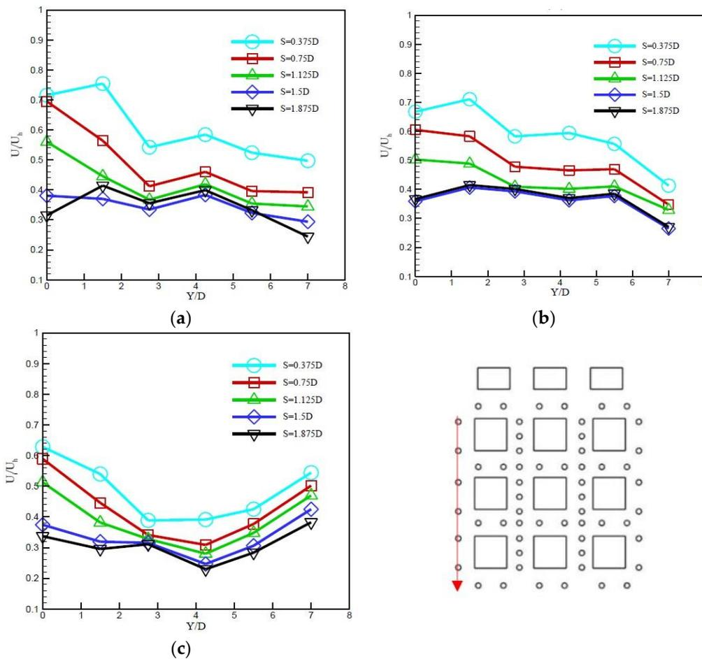
**Figure 8.** Variation of Vel in downwind street canyon L2 ( $H/D = 7$ ) (a)  $L/D = 0.75$ , (b)  $L/D = 1$  (c)  $L/D = 1.5$ .
