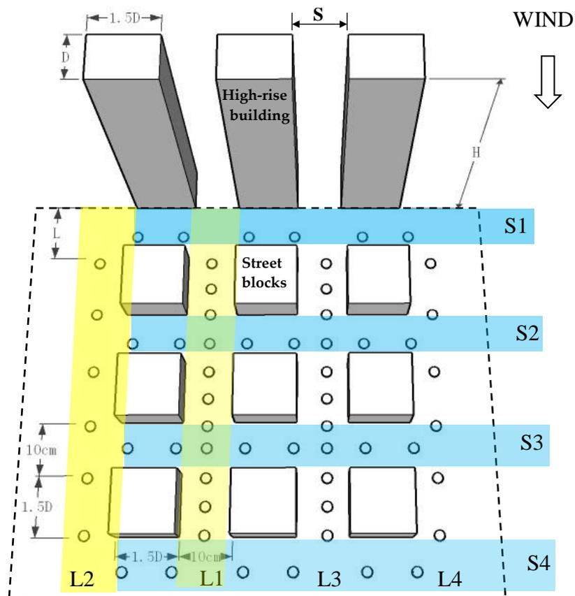
**Figure 2.** Schematic diagram of the investigated model and wind speed measurement points (Symbol O).
