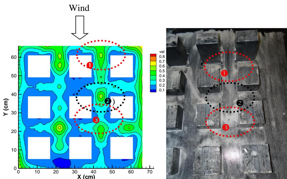
**Figure 4.** Comparison between the wind tunnel testing results (left) and the oil film observation (right) of the case  $H = 2D$ ;  $S = 1.125D$ .
