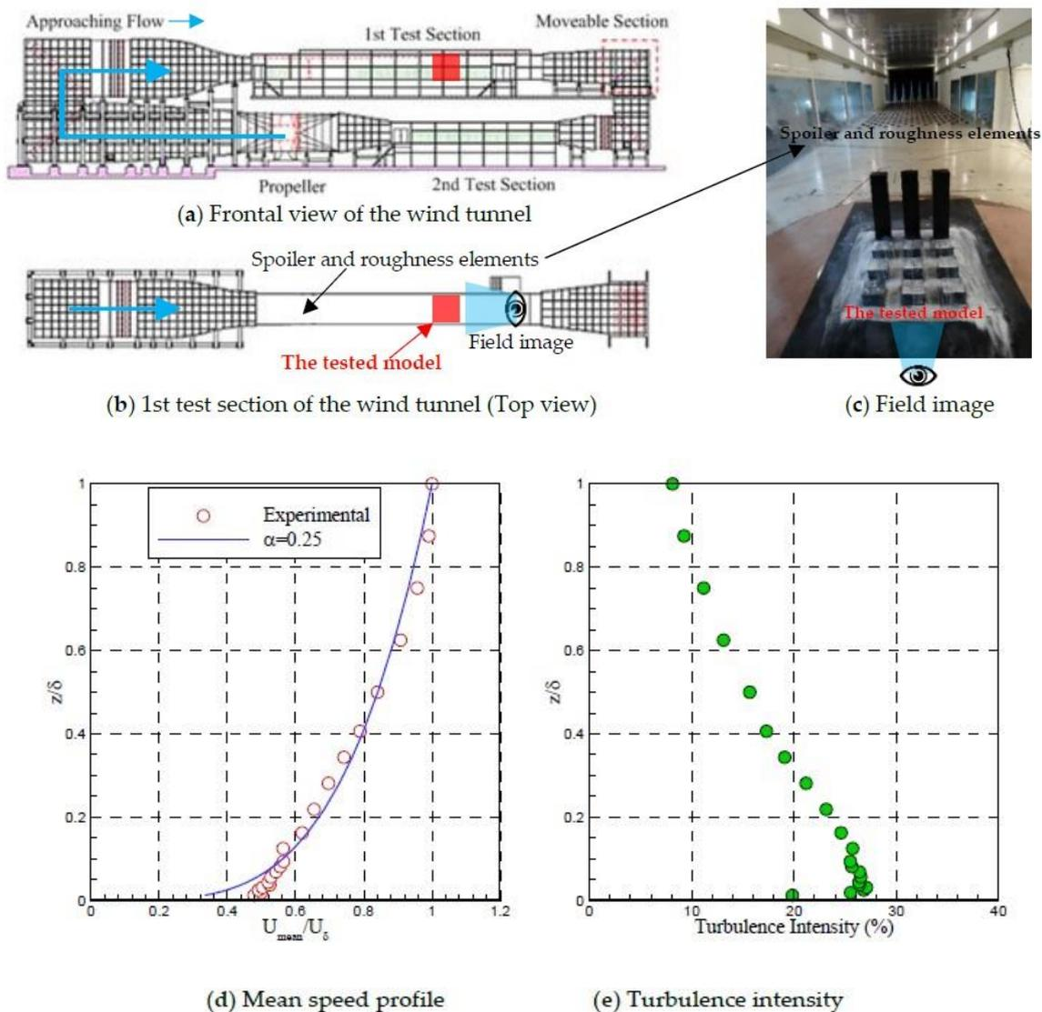
**Figure 3.** Wind tunnel and approaching wind profile [2]. (a) Frontal view of the wind tunnel; (b) 1st test section of the wind tunnel (top view); (c) field image; (d) mean speed profile; and (e) turbulence intensity.
