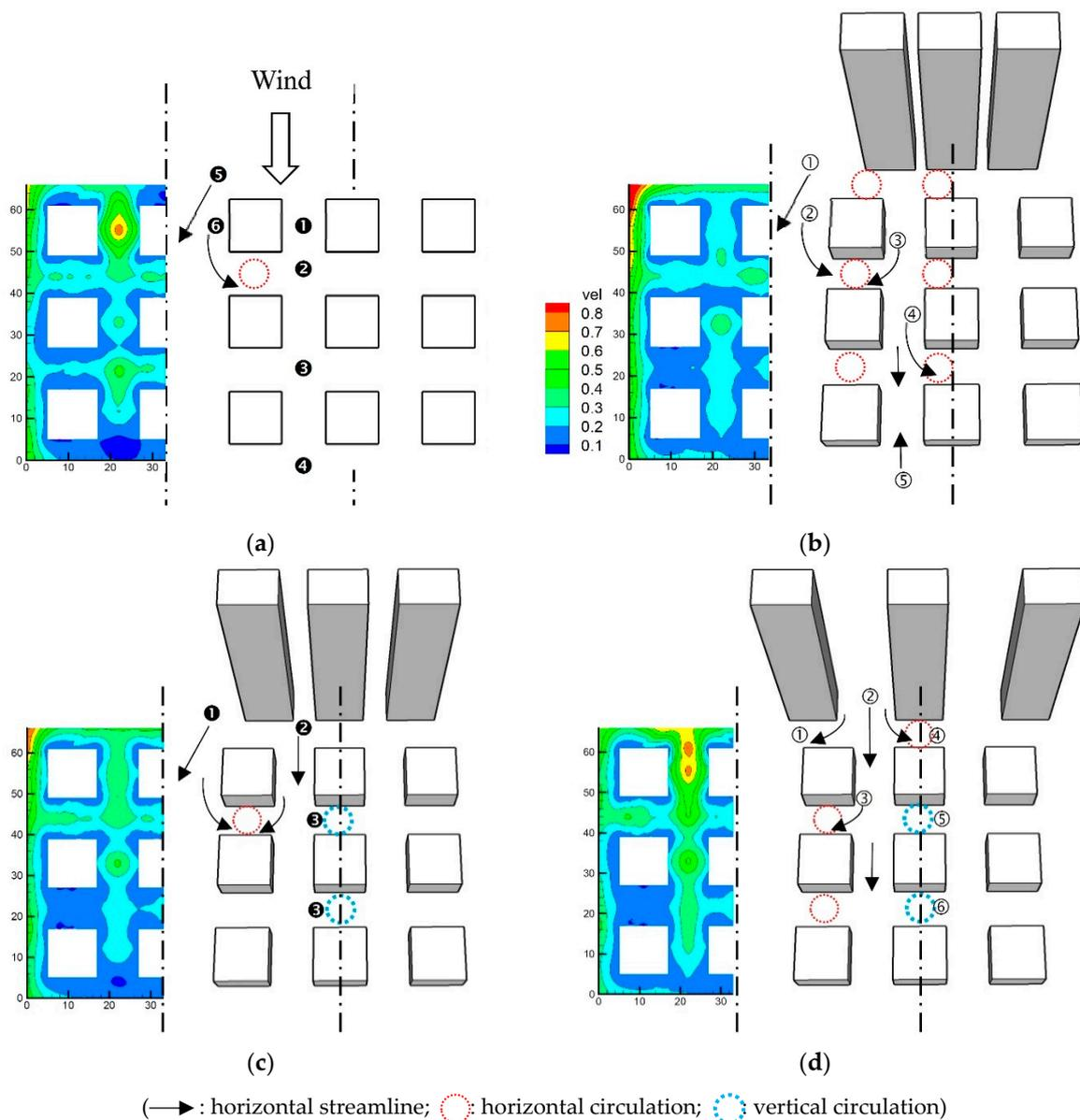
**Figure 5.** Airflow velocity (Vel) distribution in the street canyons ( $H/D = 7$ ,  $L/D = 1$ ). (a) No high-rise buildings in front. (b)  $S/D = 0.375$ . (c)  $S/D = 0.75$ . (d)  $S/D = 1.875$ .
