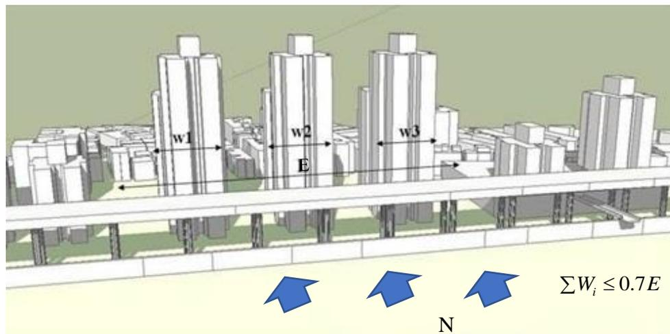
**Figure 1.** High-rise building façade width limited by the urban design specification (restricted zone on the north side of Banqiao Jiangcui in New Taipei City, Taiwan) ( $W_i$  = maximum width of the façade of each high-rise building;  $E$  = average width of the construction site).
