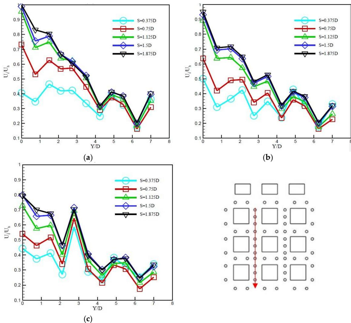
**Figure 7.** Variation of  $Vel$  in downwind street canyon L1 ( $H/D = 7$ ) (a)  $L/D = 0.75$ , (b)  $L/D = 1$  (c)  $L/D = 1.5$ .
