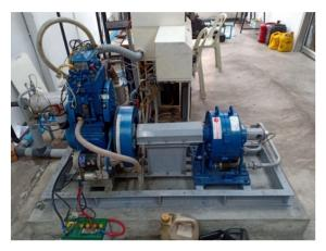
Figure 1. Experimental setup for engine testing.
