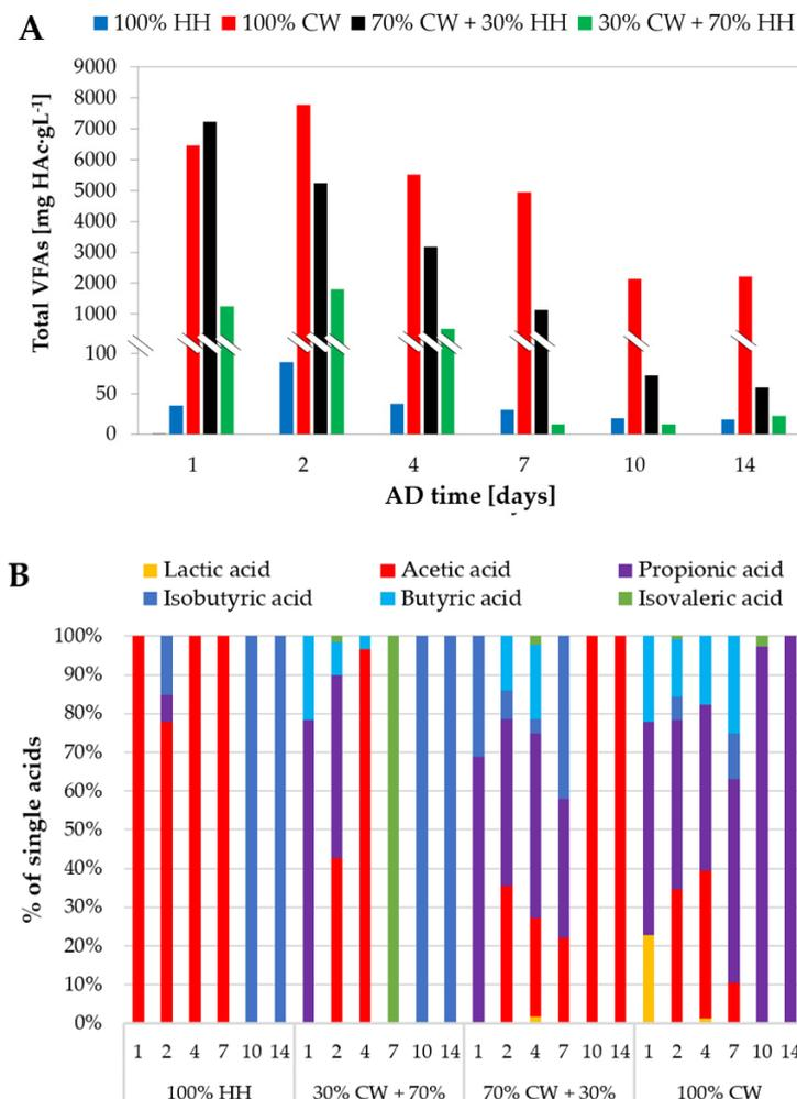
**Figure 2.** (A) Concentration of total volatile fatty acids (VFAs) as intermediates of anaerobic digestion (AD) of standalone cheese whey (CW) and hemp hurds (HH) as well as of co-digestion (coAD) of 70% CW + 30% HH and 30% CW + 70% HH. (B) Percentage of lactic acid and each VFA over the total acid concentration (calculated on an equivalent acetic acid basis) during the initial 14 days of AD and coAD.
