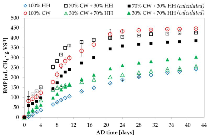
**Figure 1.** Cumulative, specific biomethane production profiles obtained along the 42 days of mesophilic anaerobic digestion and co-digestion with the four different substrate combinations tested. The filled squares and triangles indicate the calculated biomethane productions.
