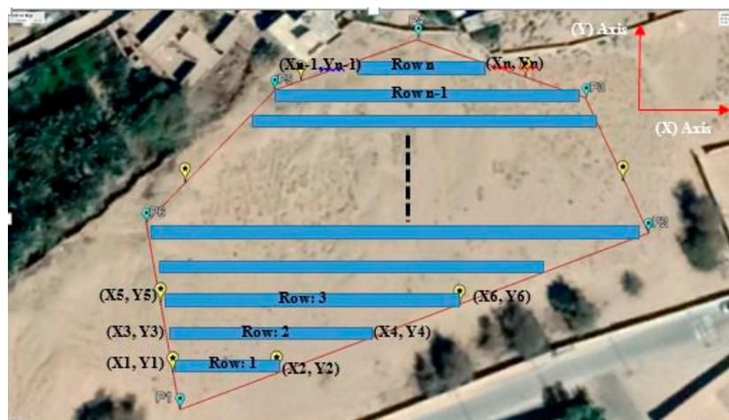
**Figure 7.** Arrangement of PV modules according to PV plant shape.
