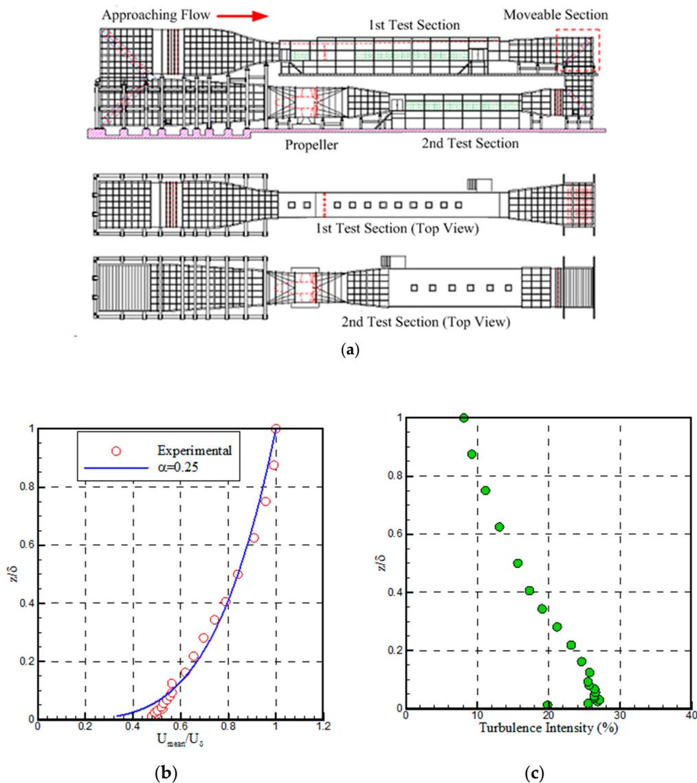
**Figure 4.** Wind-tunnel diagrams and approaching wind profile in wind-tunnel [2]. (a) Schematic (left) and photo (right) wind-tunnel; (b) mean speed profile; (c) mean speed profile.
