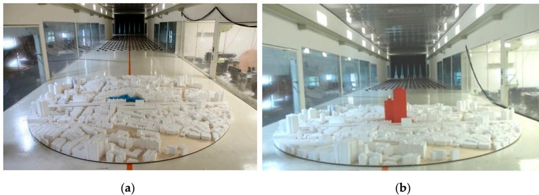
**Figure 1.** Wind-tunnel test model. (a) Before urban renewal; (b) after urban renewal.
