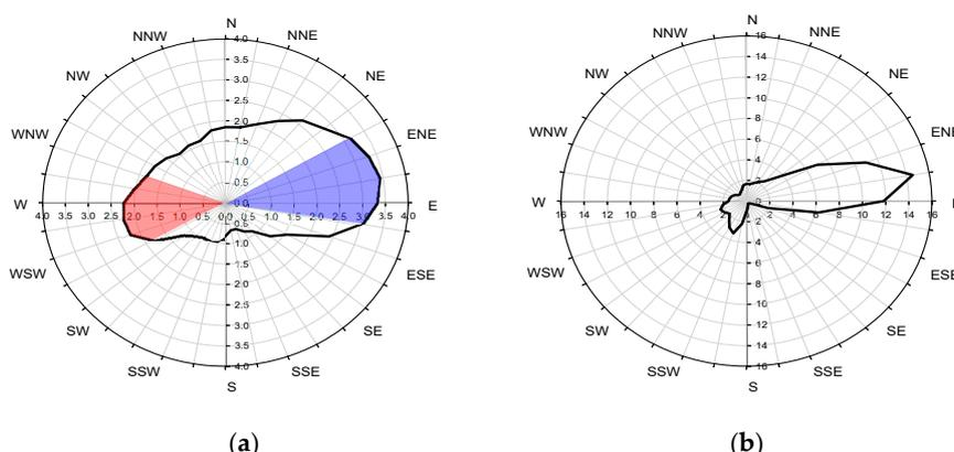
**Figure 3.** Wind speed and wind direction data acquired at meteorological stations near the urban renewal site for 2003–2013. (a) Mean wind speed for various wind directions; (b) after urban renewal probability of each wind direction.
