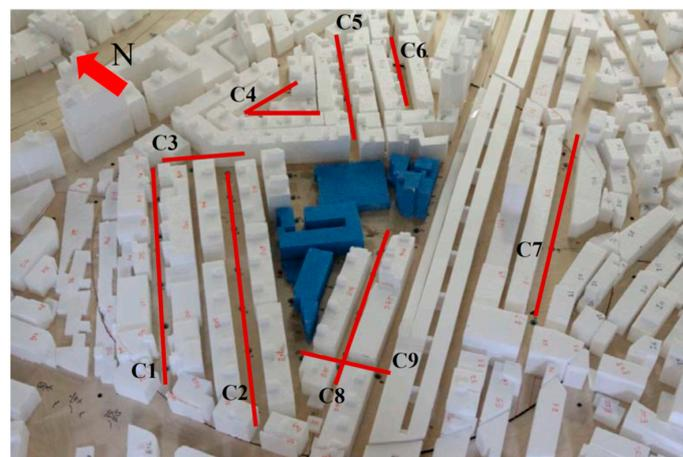
**Figure 2.** Placement of Irwin probes within street canyons C1–C9.
