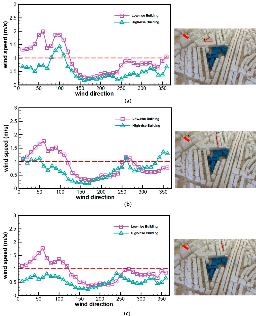
**Figure 6.** Characteristics of pedestrian wind environments in street canyons C4–C6 before and after urban renewal. (a) Street canyon C4; (b) street canyon C5; (c) street canyon C6.
