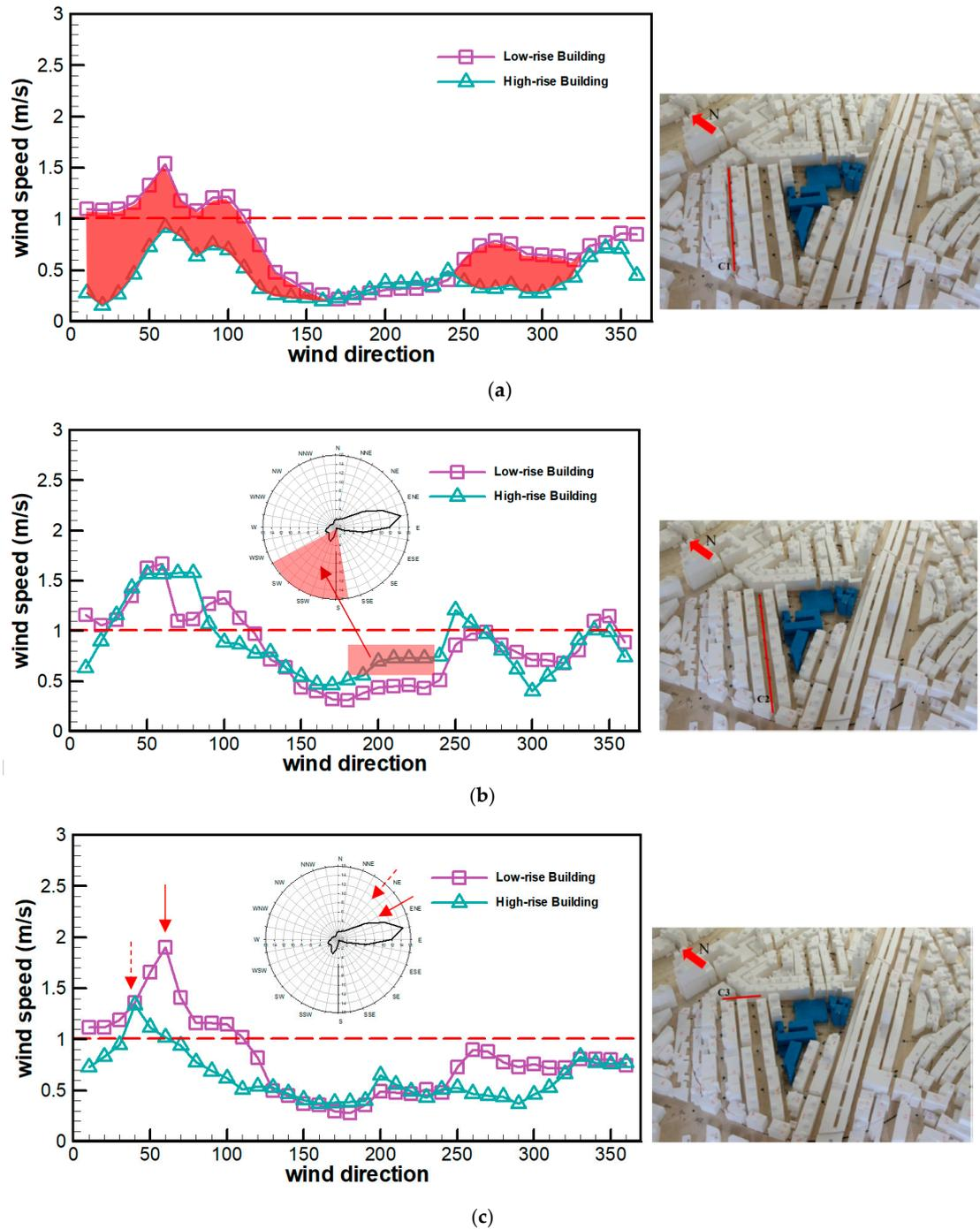
**Figure 5.** Characteristics of pedestrian wind environments in street canyons C1–C3 before and after urban renewal. (a) Street canyon C1; (b) street canyon C2; (c) street canyon C3.
