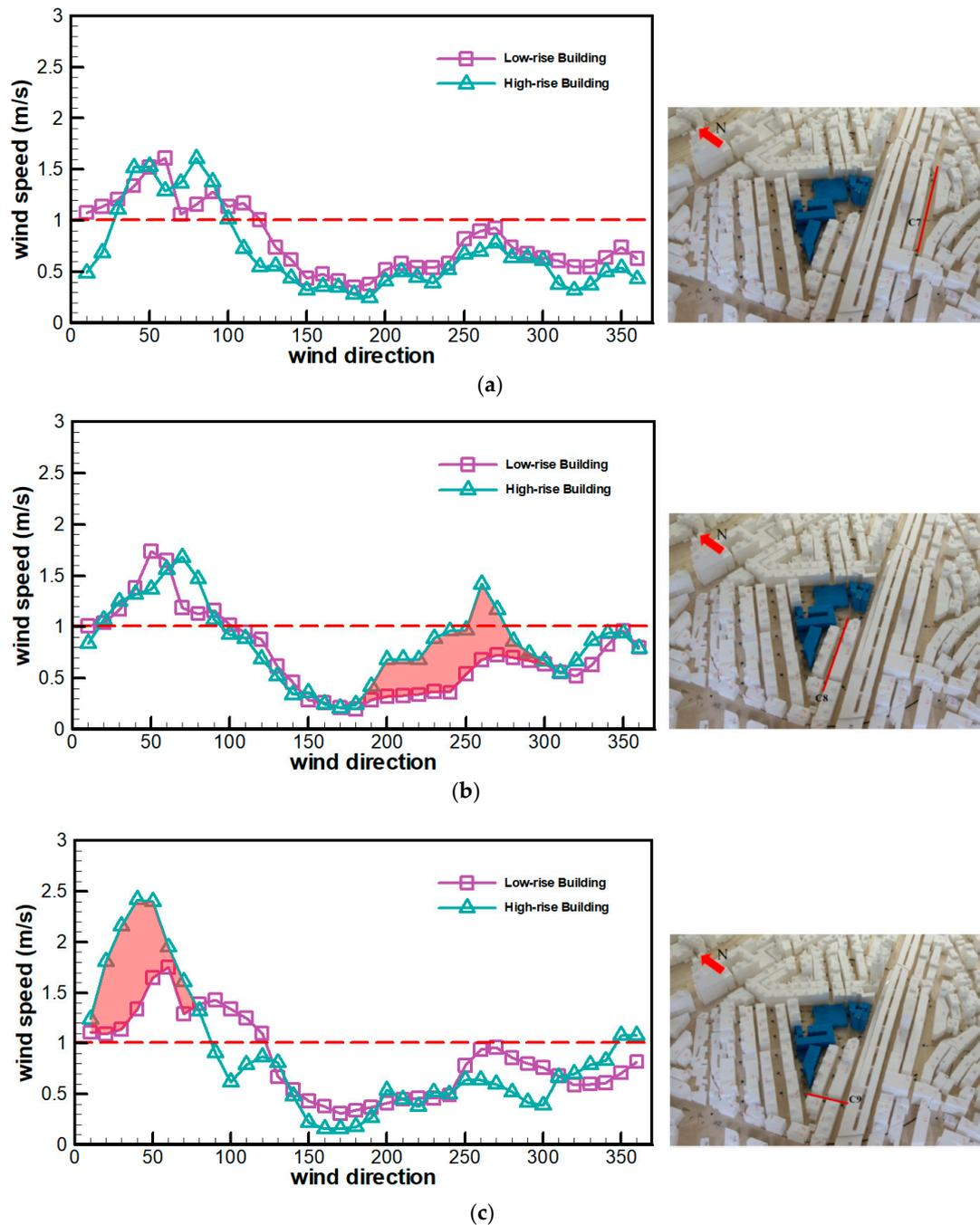
**Figure 7.** Characteristics of pedestrian wind environments in C7–C9 before and after urban renewal. (a) Street canyon C7; (b) street canyon C8; (c) street canyon C9.
