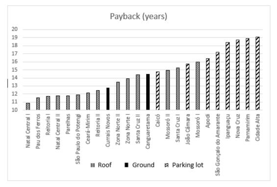
per installed kWp. As a result, the six lowest payback plants were installed on the roof, while the six highest payback plants were installed in parking lots. This analysis can be better visualized in Figure 7.
