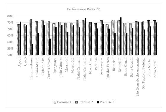
Figure 4. Performance Ratio, PR, for the IFRN-Solar project plants considering Premises 1, 2, and 3.
