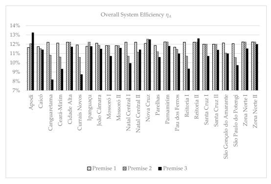
**Figure 6.** Global System Efficiency,  $\eta_A$ , for the IFRN-Solar project plants considering Premises 1, 2, and 3.
