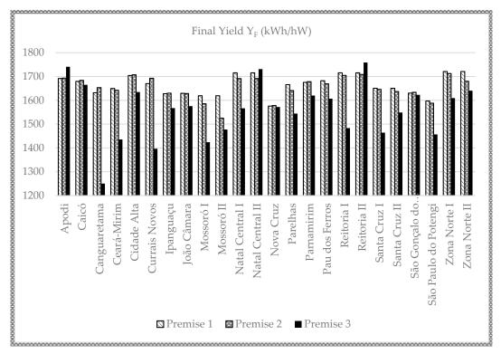
Figure 3. Final Yield, Y<sub>F</sub>, for the IFRN-Solar project plants considering Premises 1, 2, and 3.
