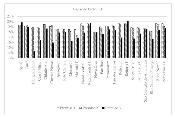
Figure 5. Capacity Factor, CF, for the IFRN-Solar project plants considering Premises 1, 2, and 3.
