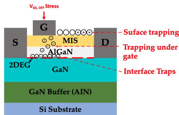
**Figure 9.** Schematic diagram of a device illustrates possible electron trapping in the GaN cascode power switch under pulsed and prolonged off-state gate  $V_{GS, OFF}$  bias stress.
