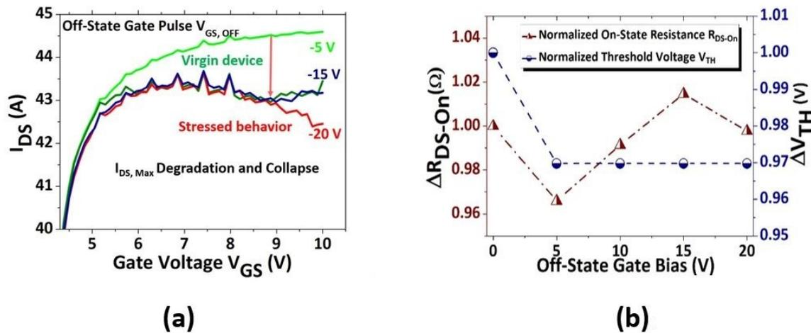
Figure 5. Results of pulsed off-state gate pulse bias on cascode 650 V power switch; (a)  $I_{DS}$  behavior under Low/Mid off-state pulsed gate bias stress, and (b) minimal and recoverable  $\Delta R_{DS-ON}$  degradation and  $\Delta V_{TH}$  shift with off-state gate bias.
