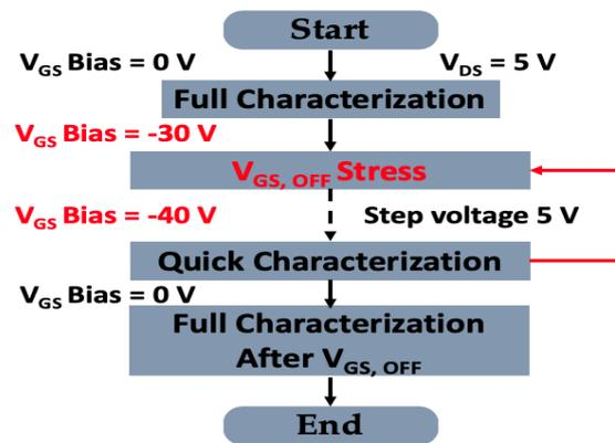
Figure 4. Schematic flow chart of prolonged off-state gate ( $V_{GS, OFF}$ ) bias experiment.
